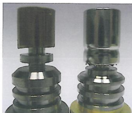
Figure 2: Transducer S8 with film (left picture) and stainless steel encapsulated (right picture) wet protector
