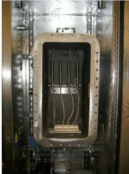
**Figure 4 Electrically heated vaporiser with four heating rods [10]**
