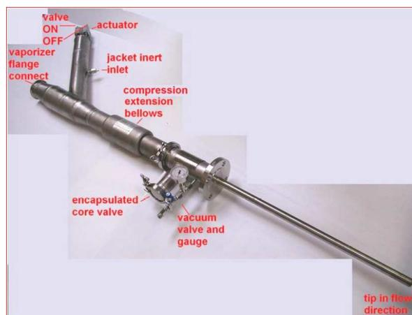
Figure 2 Vacuum insulated LNG sampling probe with connection line to vaporiser [9]
