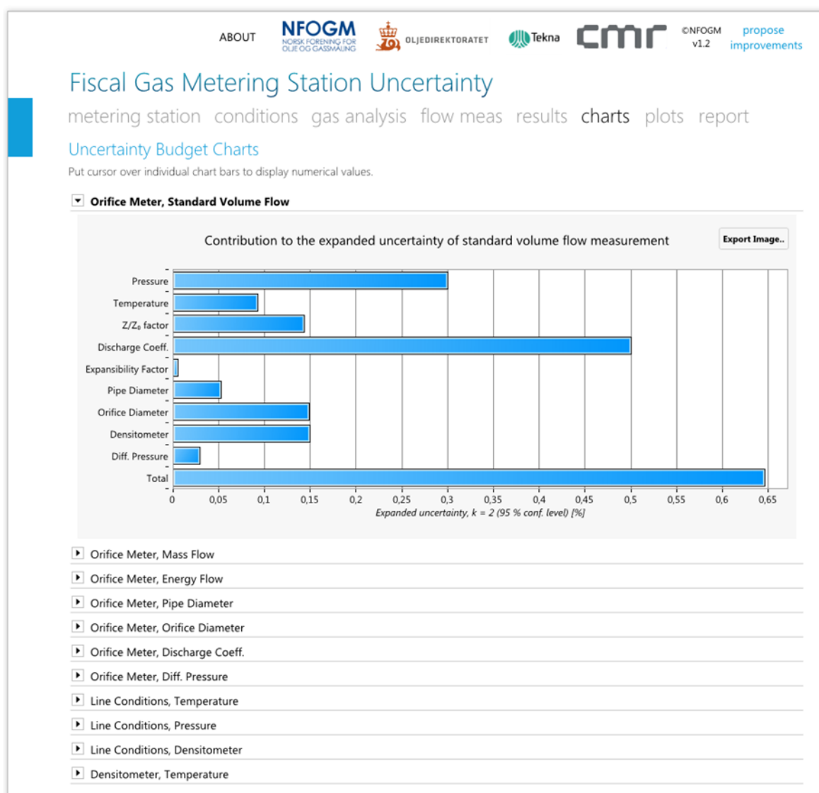
Figure 7.13 Computed uncertainty of the main flow measurement variables and equipment displayed as uncertainty budgets charts.
