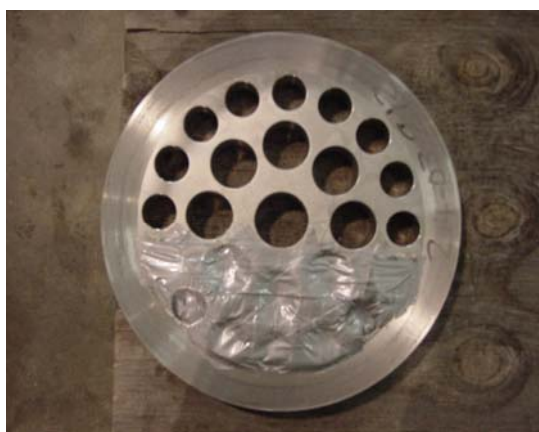
Figure 15 – Blocked Flow Conditioner
