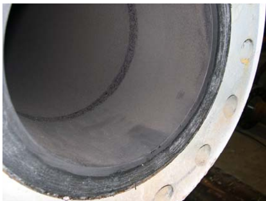
Figure 22 –Dirty Upstream Meter Tube
