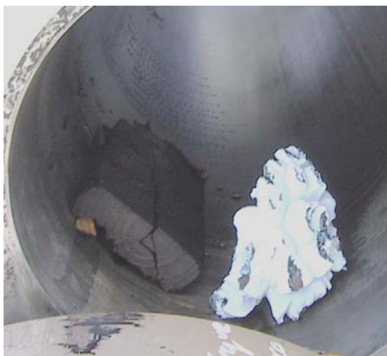
Figure 35 – 12-Inch Meter Blockage
