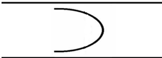
Parabolic flow profile Re < 2.000
