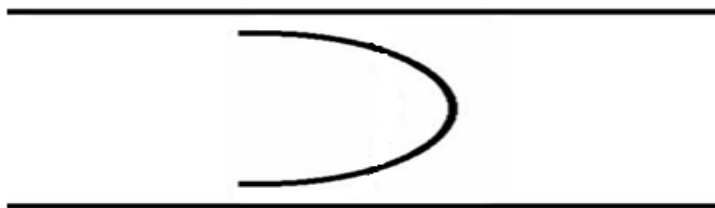
Parabolic flow profile Re < 2.000
