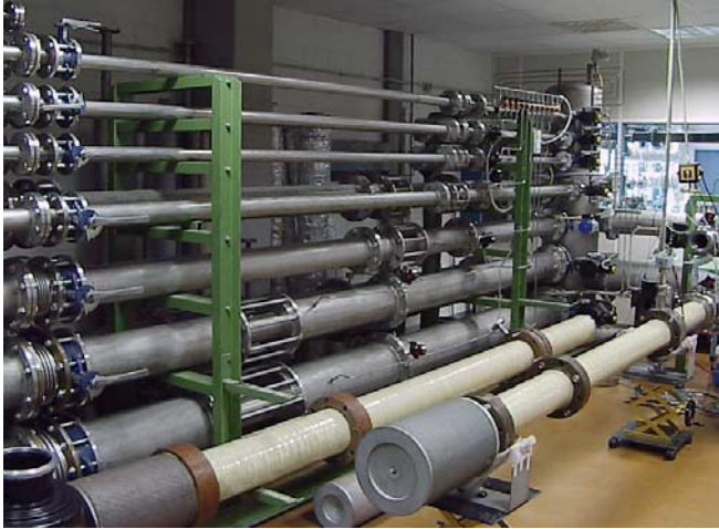
Fig. 3-17: Calibration System for Gas Flowmeters
