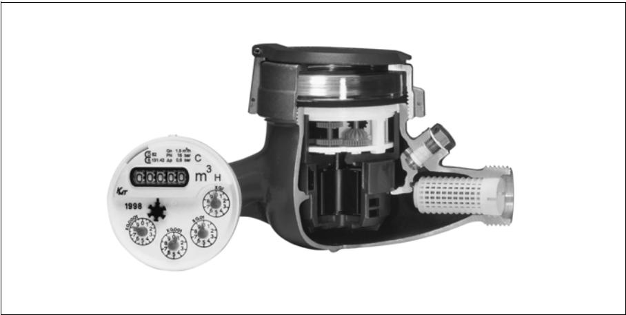
Fig. 2-15: Cross Section of a Multijet Totalizer (Type OPTIMA ARTIST)
