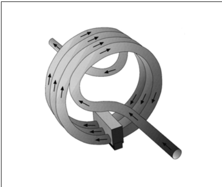
Fig. 2-107: Bent Single Tube Design
