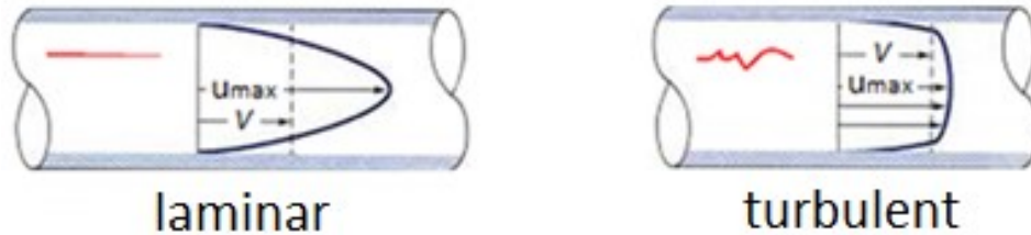
Fig 1. Influence of Reynolds Number on Flow Profile which has Knock-On Effect on Meters.
