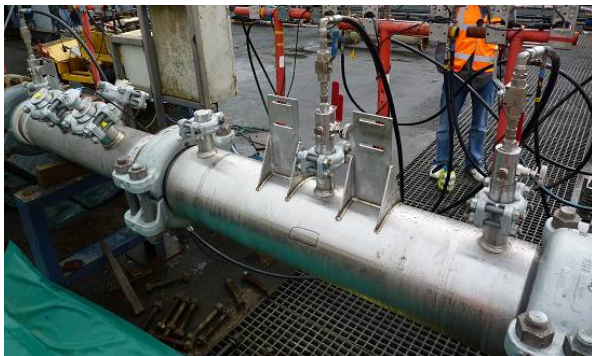
Fig 36. 10” Venturi Meter Under Calibration
