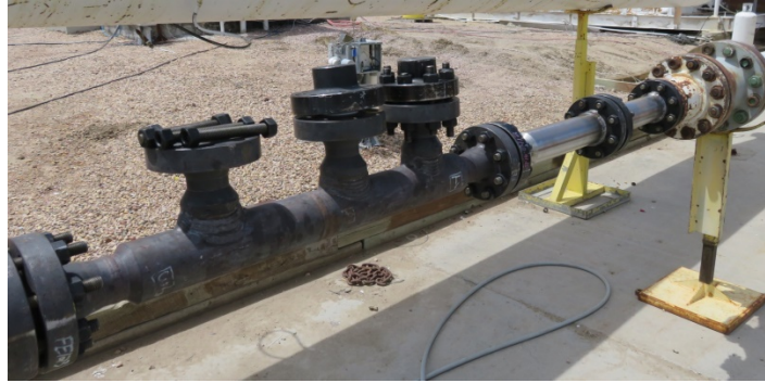
Fig 32. One of a Batch of Forty 2", 0.45 \beta Cone Meters at CEESI
