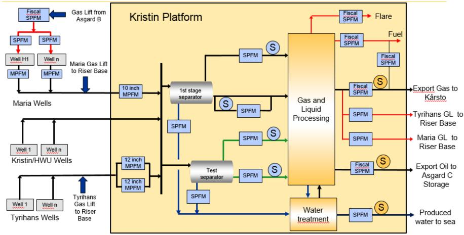
MPFM= Multiphase flow metering SPFM= Single phase flow metering
