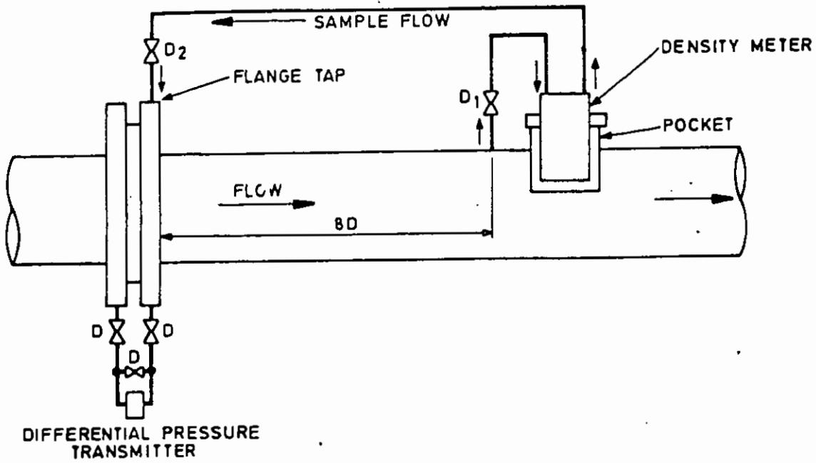
INSTALLATION OF GAS DENSITY METER ON AN ORIFICE PLATE SYSTEM USING THE PRESSURE RECOVERY METHOD
