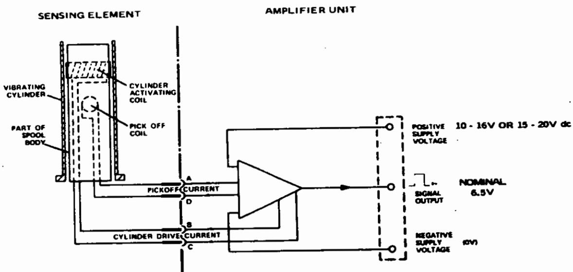
FIG. 3 Schematic Block Diagram of Transducer Circuit.
