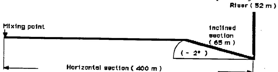
In 1986 the horizontal section of the test pipe will be reconstructed to allow for small deviations from the horizontal ( $1^\circ$  and  $1/2^\circ$  up and down) over the full pipe length ( approximately 350 meters ) .
