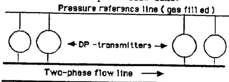
Pressure taps and transmitters must lay in the same horizontal plane.
