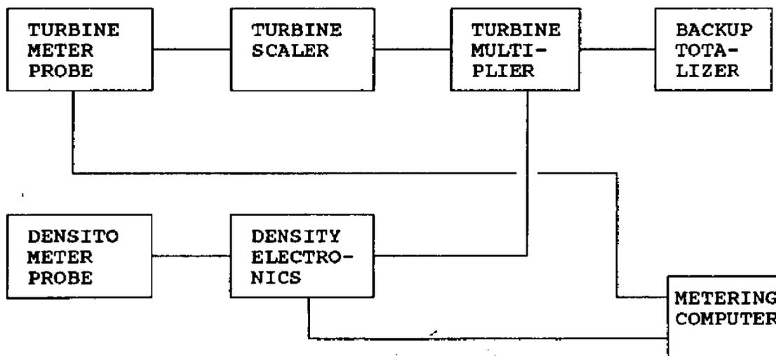
Figure 1 Block diagram of flare metering system on Ekofisk
