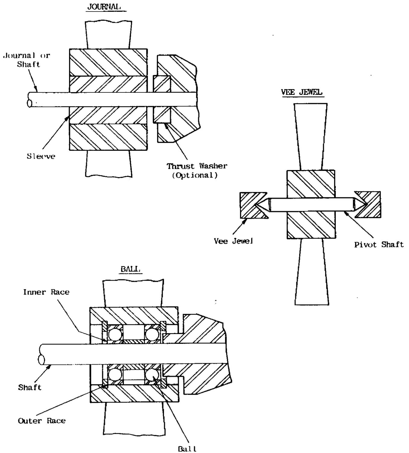
Figure 2 Bearing types used for turbine flowmeter
