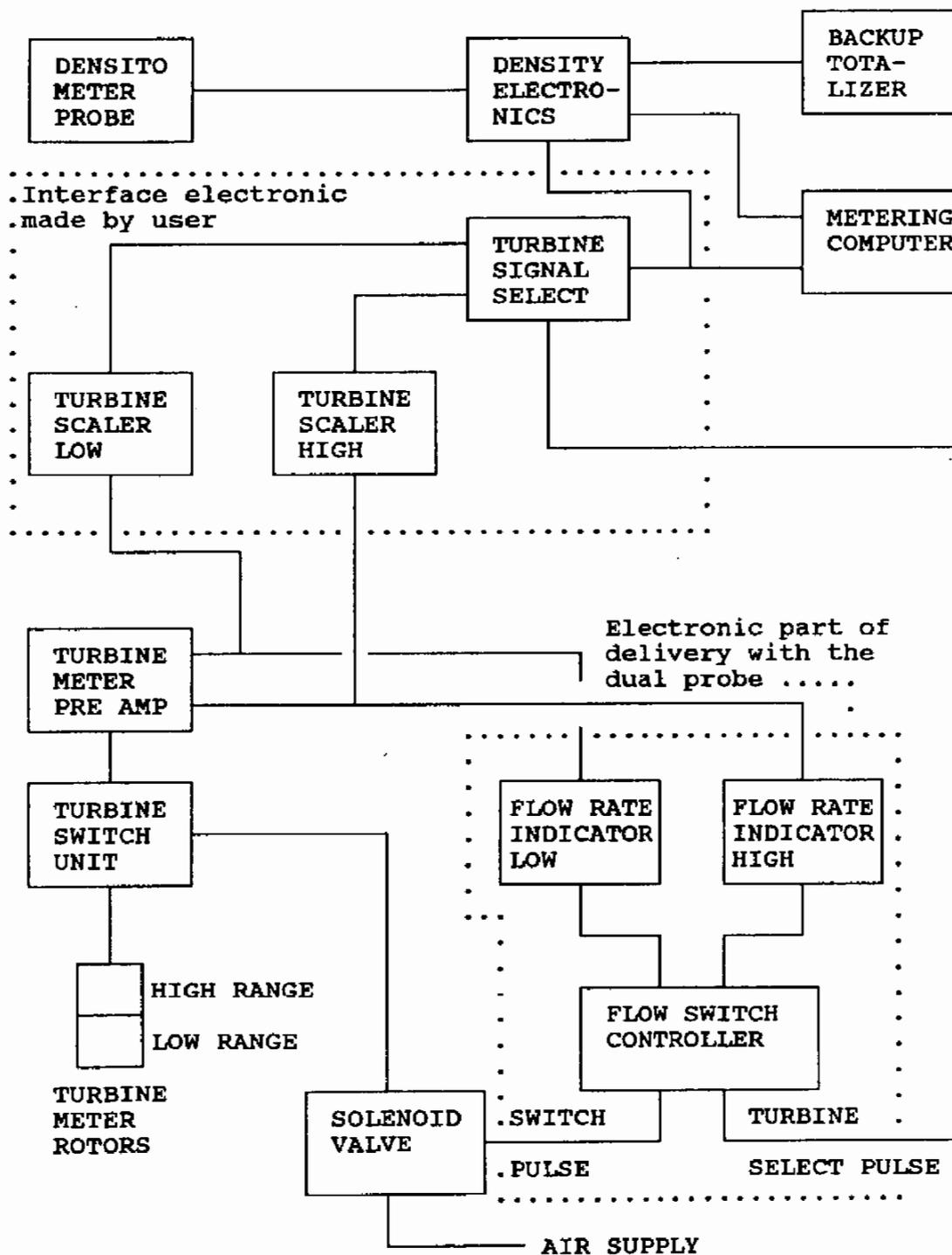
Figure 4 Principle Interface of dual flare probe
