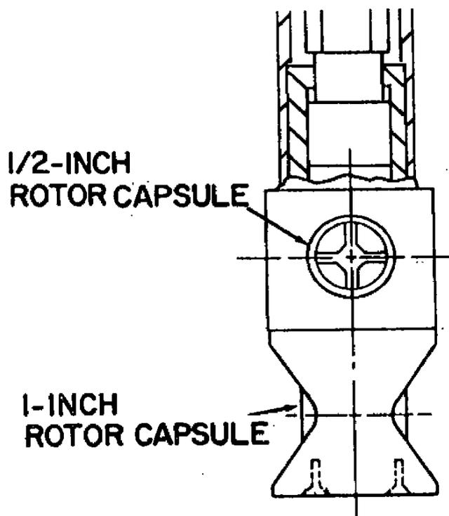
Figure 3 Dual flare probe rotor assembly
