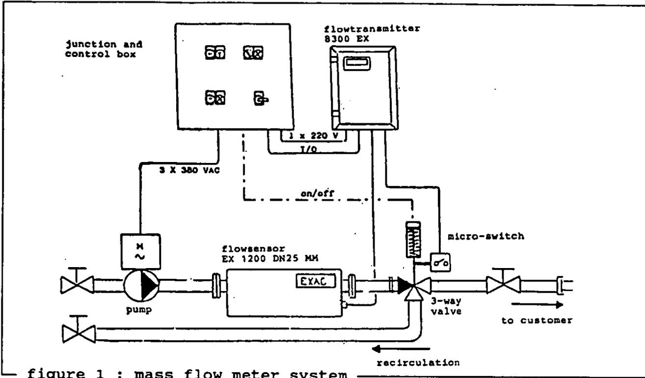
figure 1 : mass flow meter system
