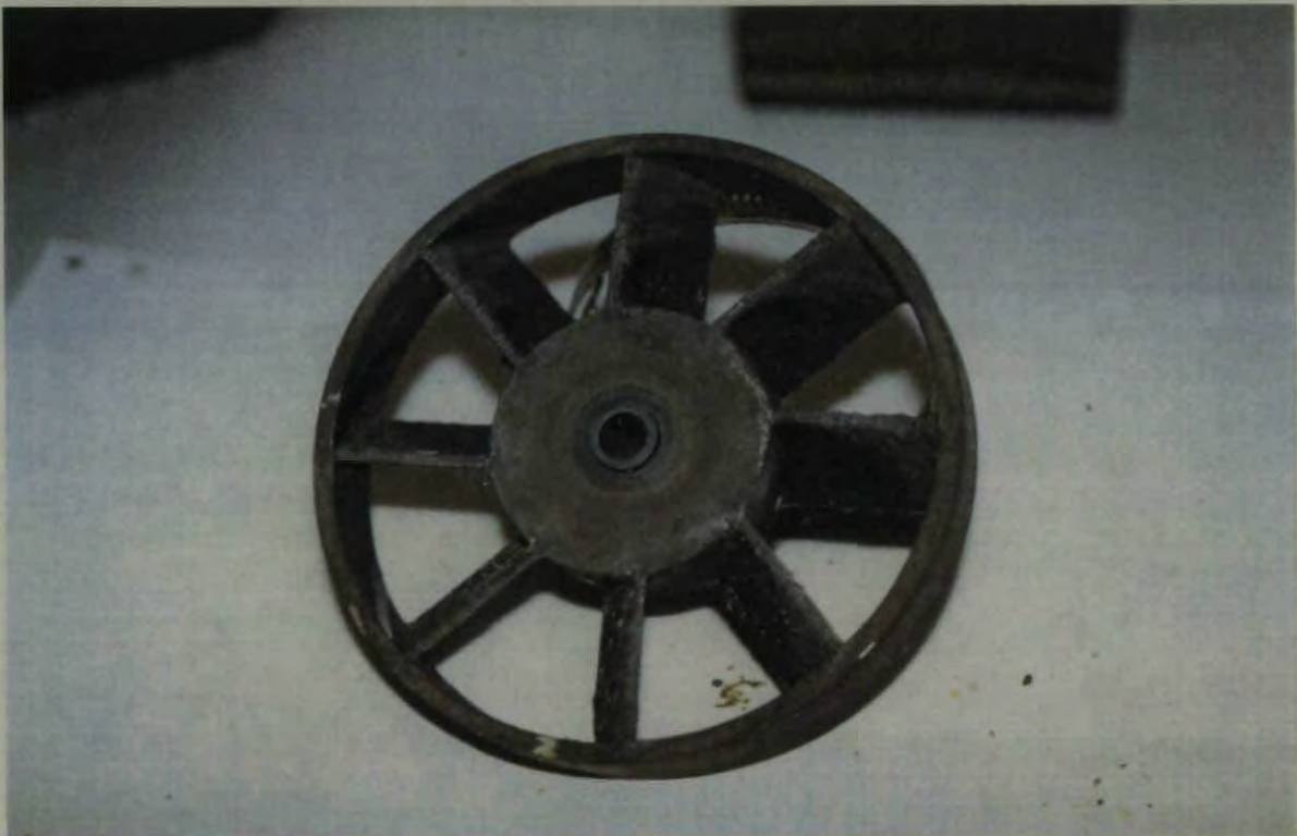
Figure 9. Scale deposits on impeller of turbine meter.
