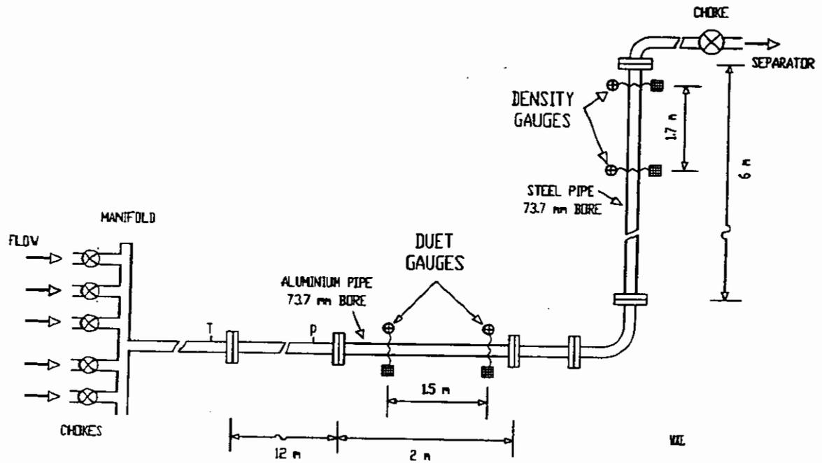
Figure 2. Schematic of the test pipeline joining the manifold and the test separator on the Vicksburg platform. P and T indicate pressure and temperature transducers.
