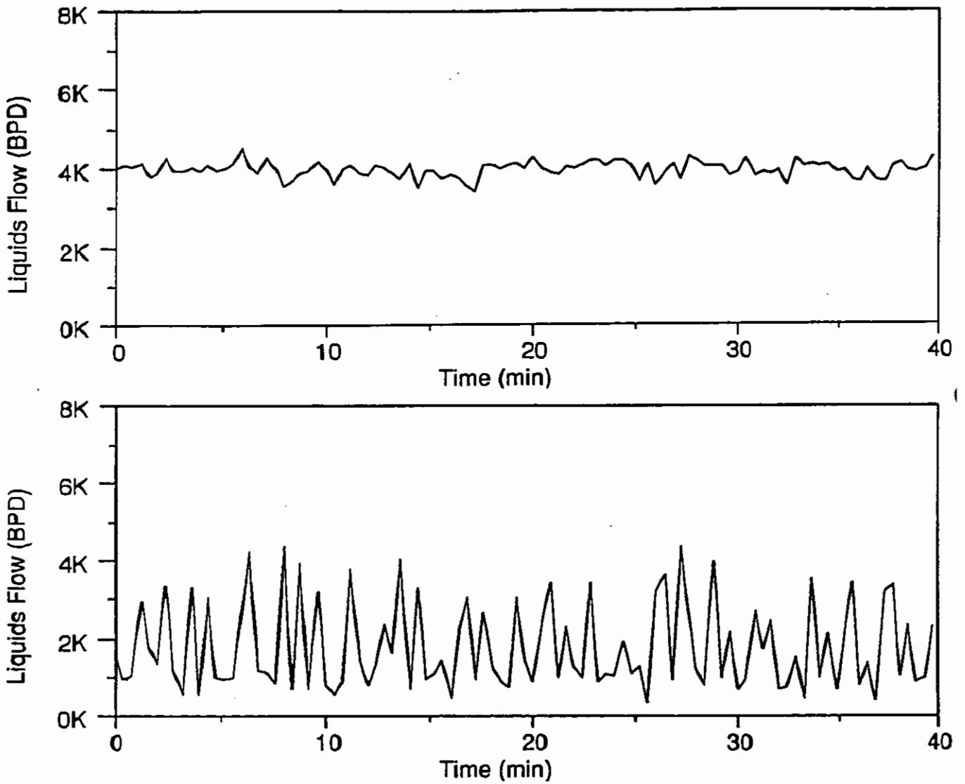
Figure 6. Variation of the volume flow rate of the liquids (oil + water) with time for the flow of SP7 and SP4 wells in the vertical section of the test pipeline.
