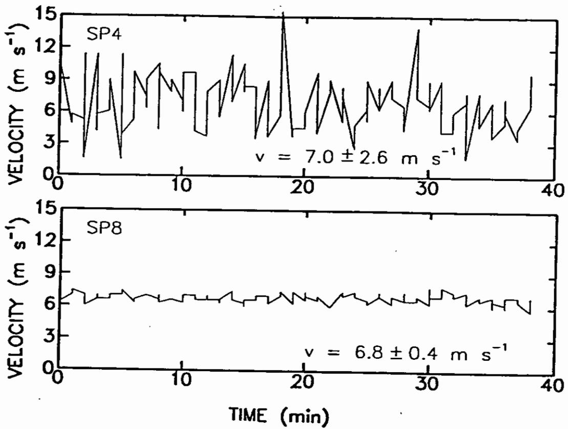
Figure 5. Velocity versus time for the flows from the SP4 and SP8 wells, determined by cross-correlation averaged over 17 second periods.
