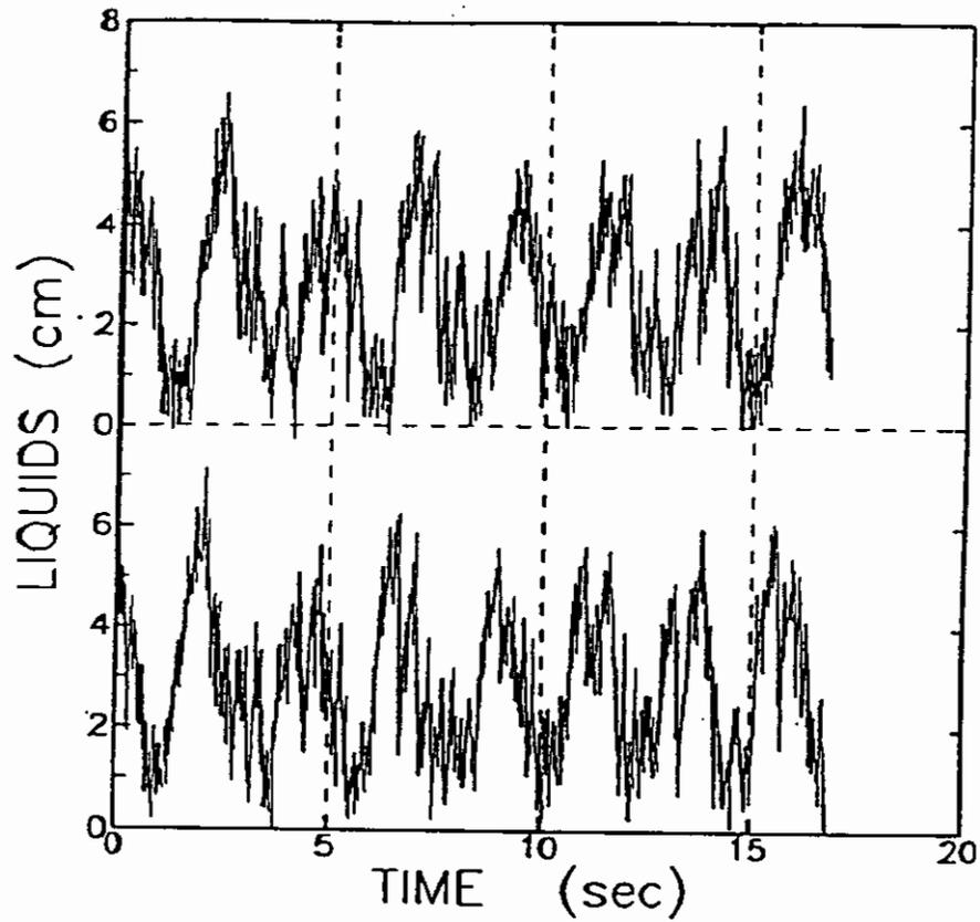
Figure 4. Variation in mass per unit area of liquids (in the gamma-ray beam) with time for the two gauges mounted on the vertical pipeline. The time delay between the upstream gauge (lower record) and upstream gauge is 0.4 seconds.
