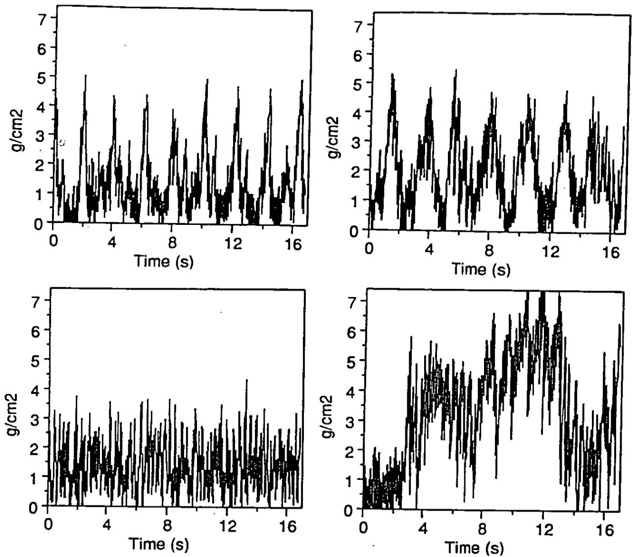
Figure 3. Variations of mass per unit area of liquids in the gamma-ray beam with time, for the flows for the SP7 well at two different pressures (top left and right), for the combined flows from the SP5 and SP6 wells (bottom left), and for the SP4 well (bottom right), in the vertical section of the test pipeline.
