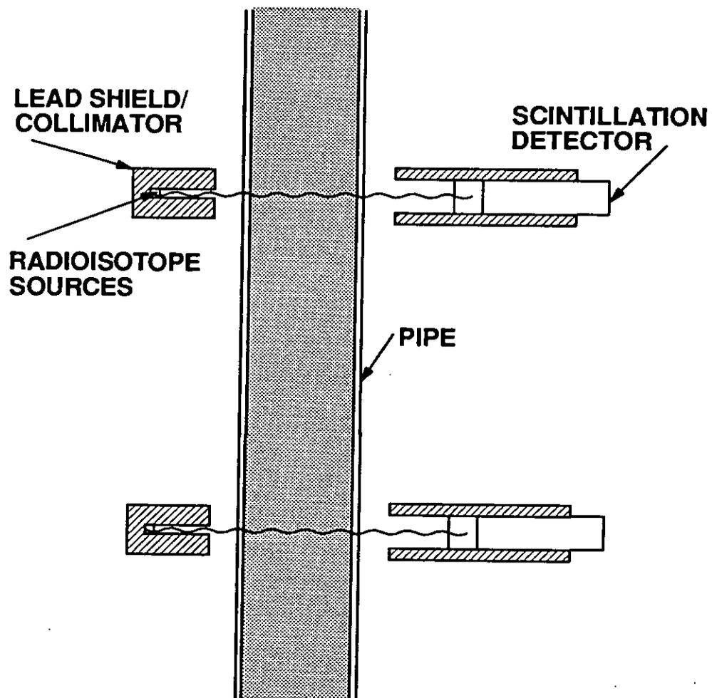
Figure 1. Gamma-ray transmission gauges mounted about pipeline.
