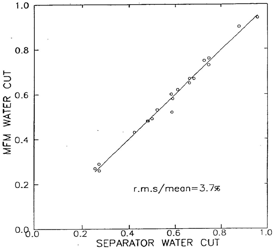
Fig. 8. Water cut for the gamma-ray MFM mounted about the vertical upflow pipeline: Phase 2 of the trial.
