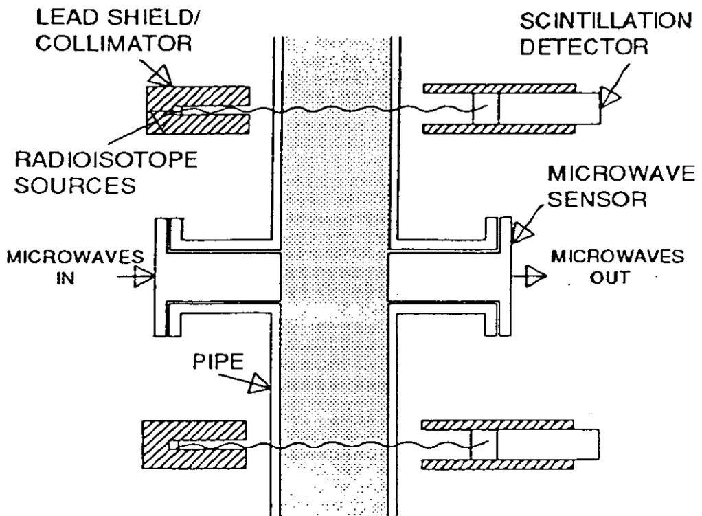
Fig. 2. Schematic of the prototype microwave/gamma-ray MFM used in the trial on Thevenard Island.
