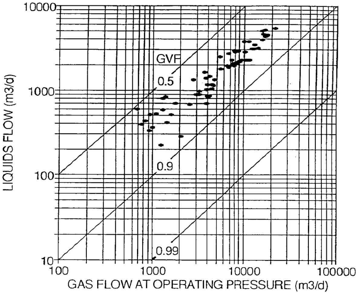
Fig. 12. Flow rates of liquids and gas (at operating pressure in pipeline) during the Vicksburg platform and Thevenard Island trials.
