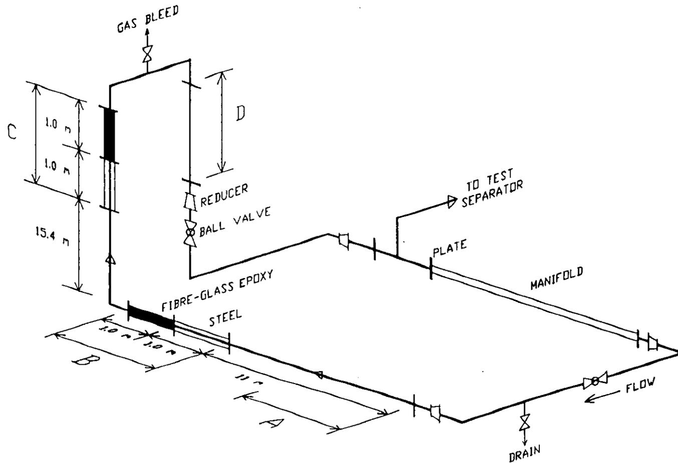
Fig. 4. Schematic of the test pipeline at Thevenard Island. A, B, C, and D are the positions at which the two-gamma-ray multiphase flow meters were mounted during the trial, with one MFM always in position C.
