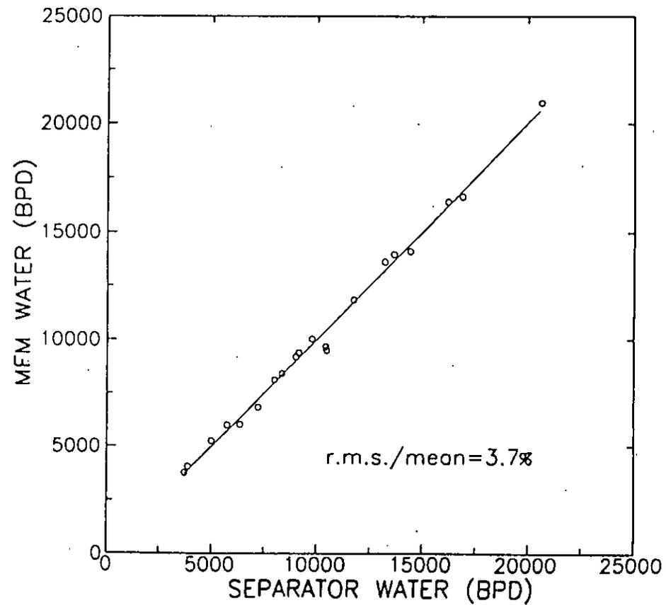
Fig. 11. Oil and water flows for the gamma-ray MFM mounted about the vertical upflow pipeline: Phase 2 of the trial.
