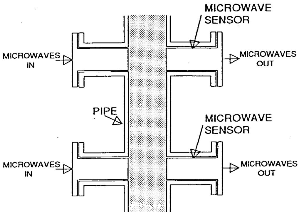
Fig. 13. Schematic of the prototype microwave MFM to be used in the West Kingfish platform trial.
