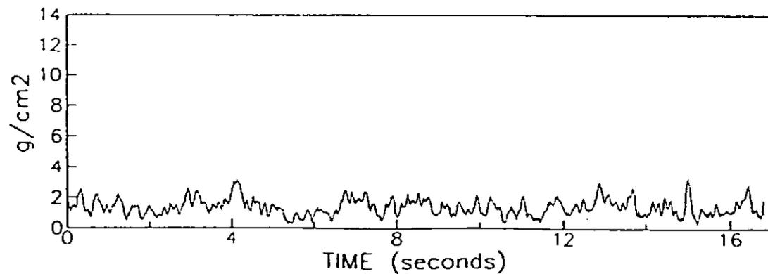
Fig. 5. Mass per unit area ( $\text{g cm}^{-2}$ ) of fluids versus time for the flow of the Saladin 4 well (top), for the commingled flow of the Saladin 4 and 5 wells (second from top), and for the commingled flow of the Saladin 7 and Yammaderry 2 wells (bottom two).
