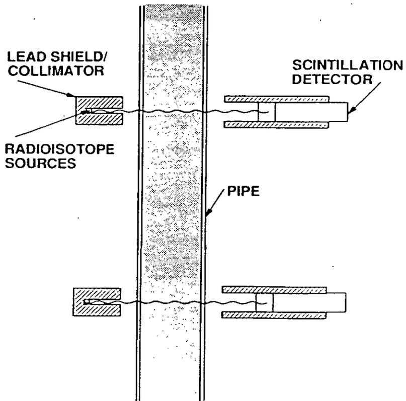
Fig. 1. Schematic of the gamma-ray MFM.
