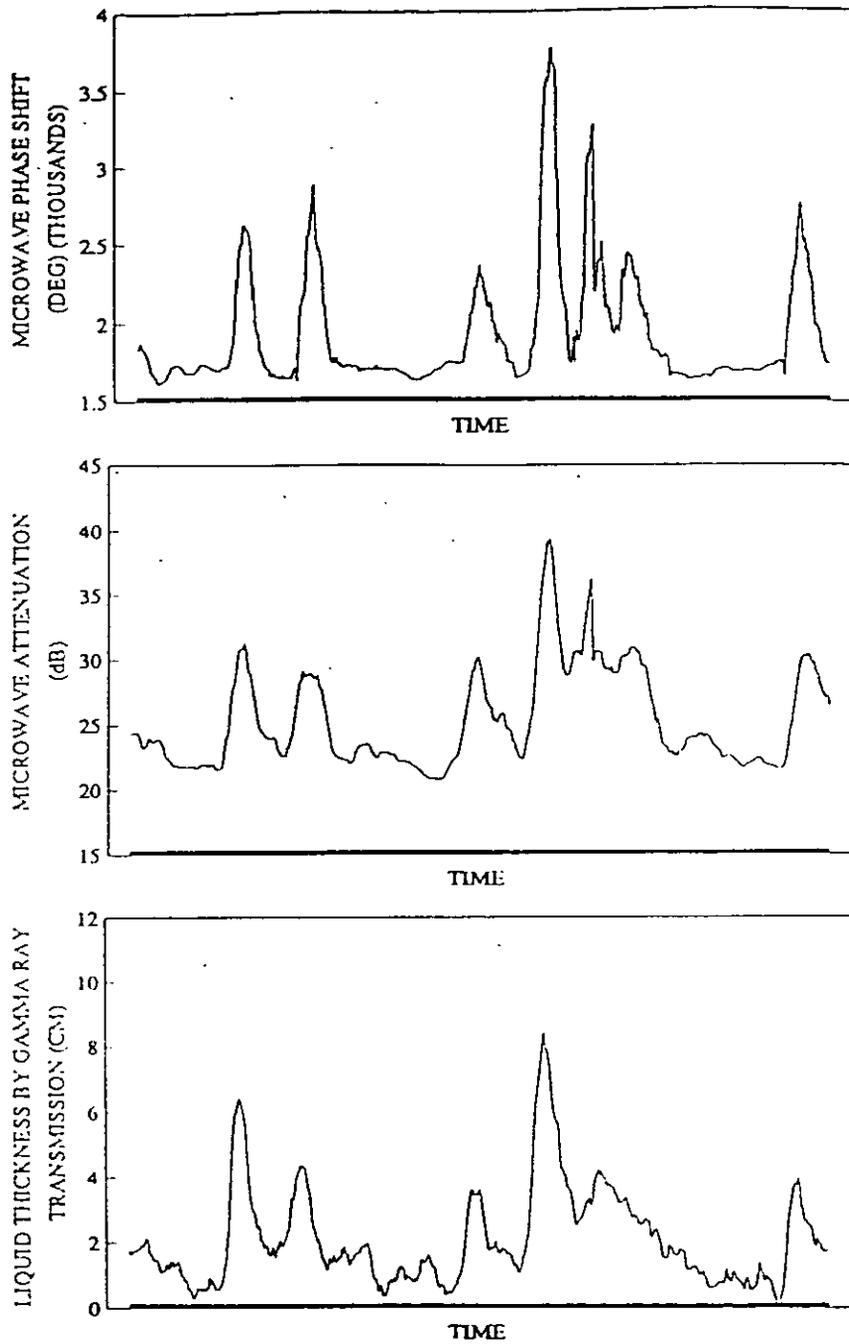
Fig. 9. Plot of microwave/gamma-ray MFM data for an ~14 s logging period of a commingled (Saladin 6+Saladin 7+Yammaderry 2) well flow during the Thevenard Island trial. The phase shift and attenuation data were measured by the microwave gauge of the MFM and liquids thickness by the gamma-ray gauge of the MFM.
