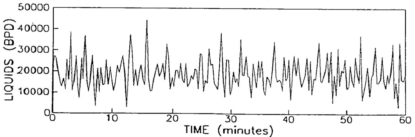
Fig. 6. The flow rate of liquids versus time for the flow from the Saladin 4 well (top), for the commingled flows of the Saladin 4 and 6 wells, and for the commingled flows of the Saladin 7 and Yammaderry 2 wells.
