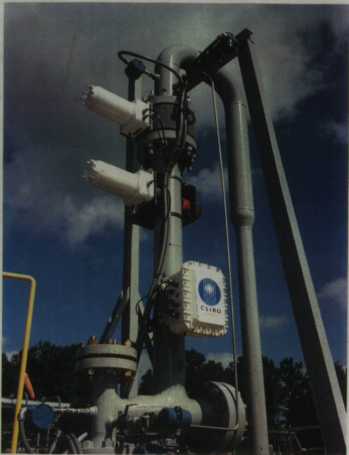
Figure 2. Photograph of the CSIRO MFM mounted on a pipeline at the Humble facility.
