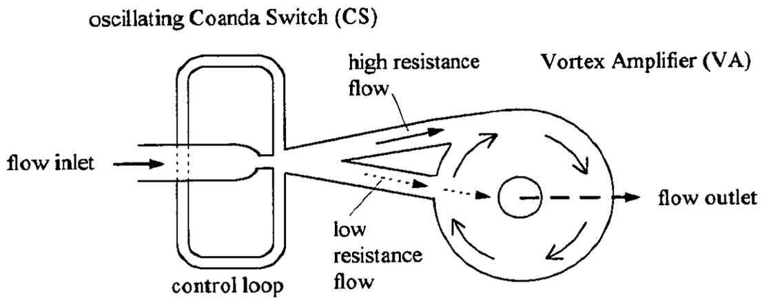
Fig.11. Traditional shape of Vortex Amplifier (VA)
