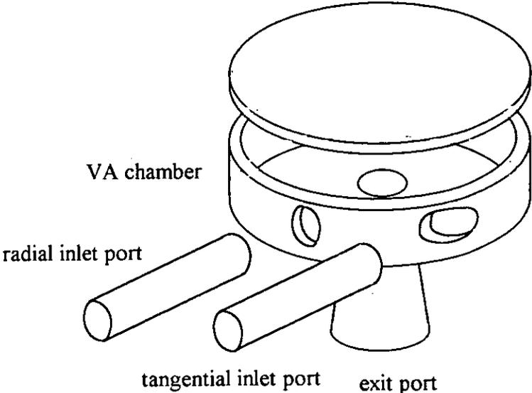
Fig. 12. Off-centred port in-line VA
