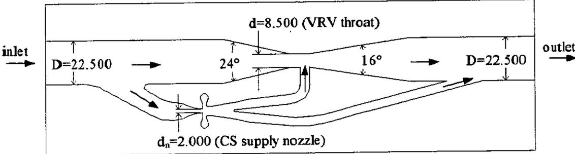
Fig.3. Measure static performance of BV flowmeter for water
