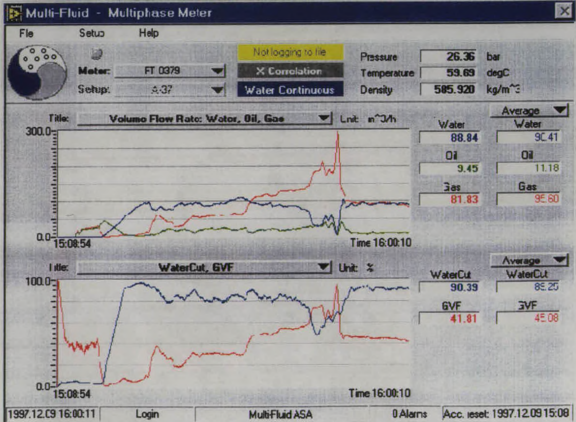
Figure 3 - Multiphase meter response for re-start of Brage well A-37
