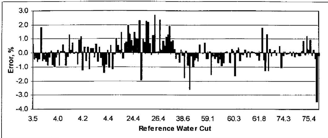
Figure 9 Water-Cut Accuracy
