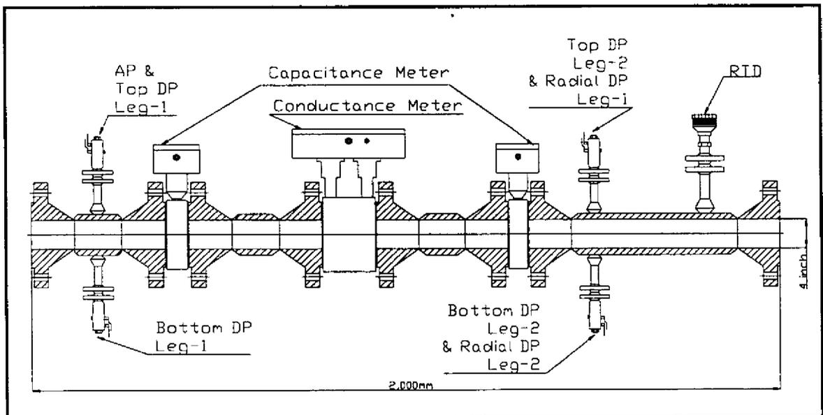
Figure 4 GA Drawing of Spool Piece
