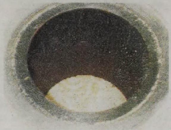
Figure 6 - O-ring after removal
