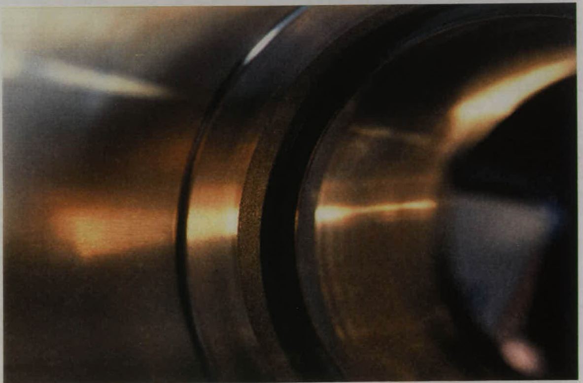
Fig 19 MANUFACTURER C. 100 mm DIAMETER METER, METER BORE WEAR
