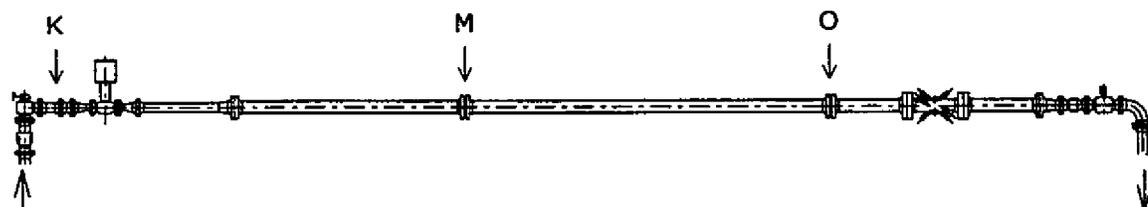
Figure 3: Test Set-up With Regulator Upstream and USM's at Long Distance (UP-L)
