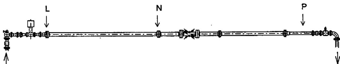
Figure 2: Test Set-up With Regulator Upstream and USM's in Middle of Test Section (UP-M)
