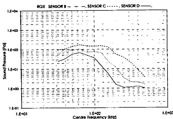
Figure 10: Results Sound Measurements Upstream of Silent Regulator RQX
