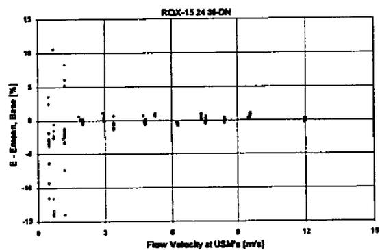
Figure 18: USM's Meter Error Shifts Upstream of Silent Regulator RQX
