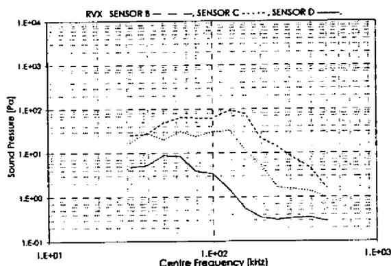
Figure 8: Results Sound Measurements Upstream of Non-Silent Regulator RVX
