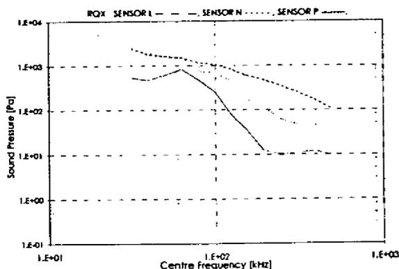
Figure 11: Results Sound Measurements Downstream of Silent Regulator RQX
