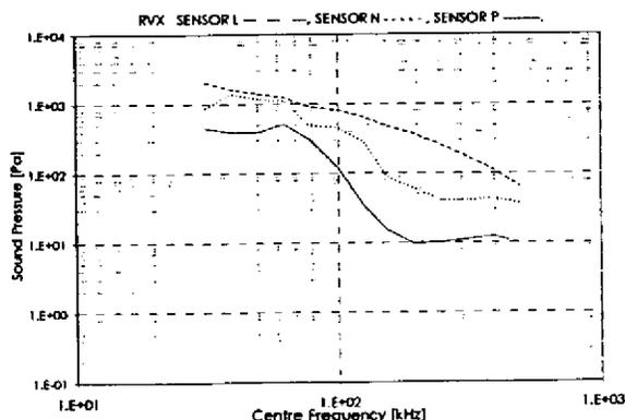
Figure 9: Results Sound Measurements Downstream of Non-Silent Regulator RVX
