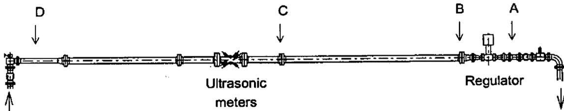
Figure 1: Test Set-up With Regulator Downstream (DN)
