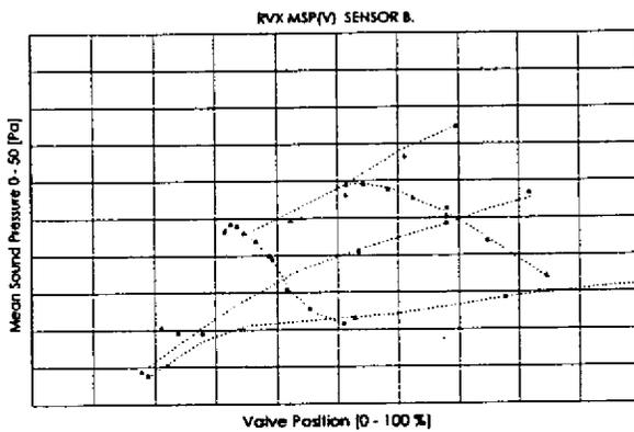
Figure 12: MSP as function of Valve Position Upstream of Non-Silent Regulator RVX
