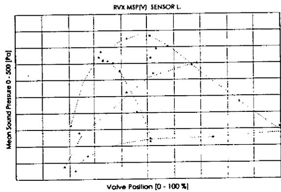
Figure 13: MSP as function of Valve Position Downstream of Non-Silent Regulator RVX
