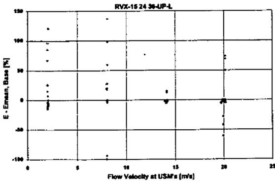
Figure 19: USM's Meter Error Shifts Downstream of Non-Silent Regulator RVX
