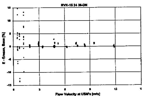
Figure 17: USM's Meter Error Shifts Upstream of Non-Silent Regulator RVX
