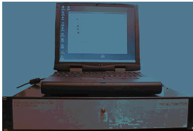
Figure 5 The prototype WLR system, including a dedicated microwave electronics unit, and a portable PC which is used to control the microwave electronics and the data collection and processing.
