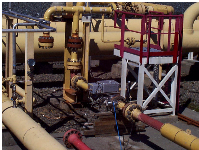
Fig. 6 Installation of a 6" MPU 1200 at Statoil's K-Lab 10D downstream a single 90^\circ bend. A flow conditioner is mounted in the read flange upstream the single bend. Photograph provided by Statoil K-Lab.
