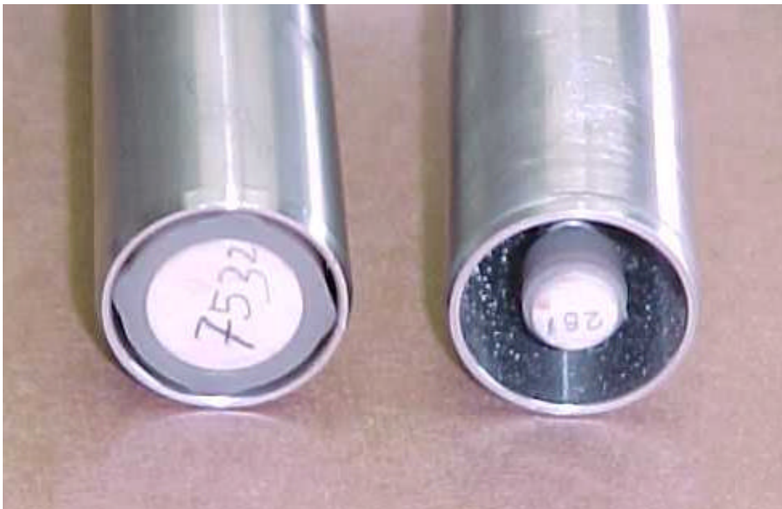
Figure 8 - Transducer tips of standard and higher frequency transducer compared
