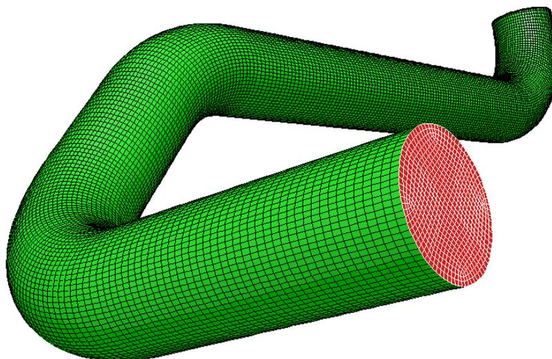
**Figure 2.** A typical section of the computational mesh used to model the pipework (between points 3 and 4 in figure 1)
