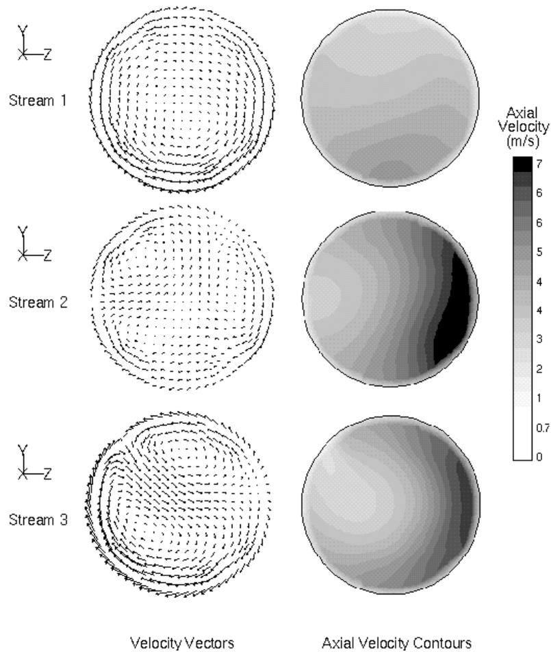
**Figure 6. Predicted Flow Behaviour 1.5m Downstream of the Header with Streams 1, 2 and 3 on-line**
