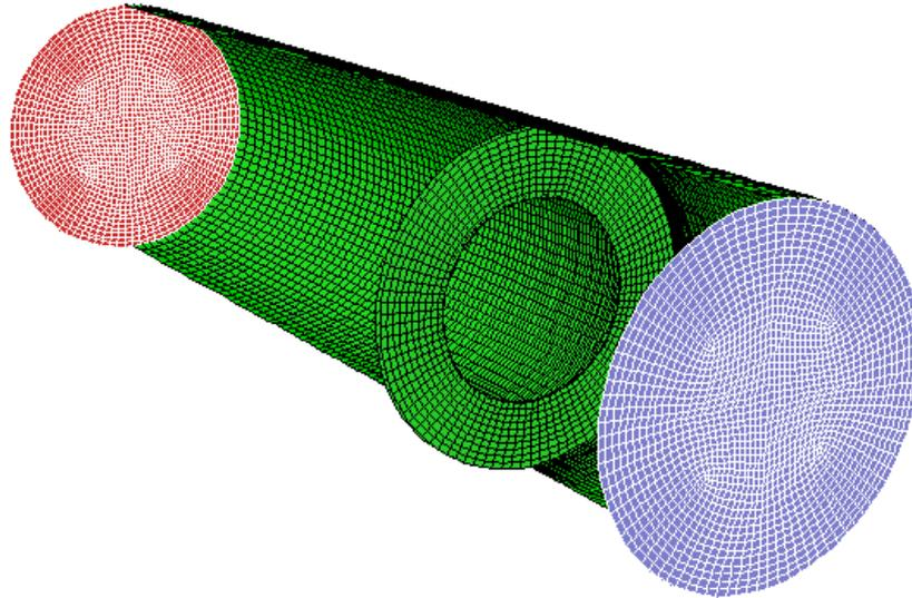
**Figure 3. The computational mesh used for modelling the orifice plate flowmeters**
