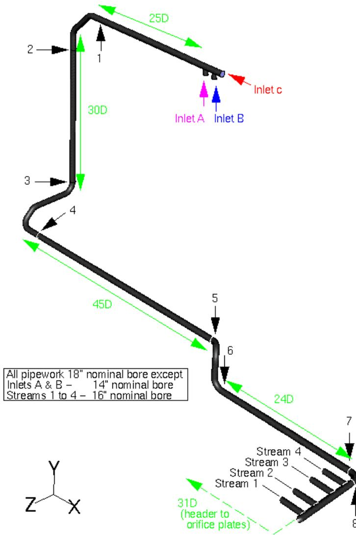
Figure 1. The Bruce Flow Metering Installation
