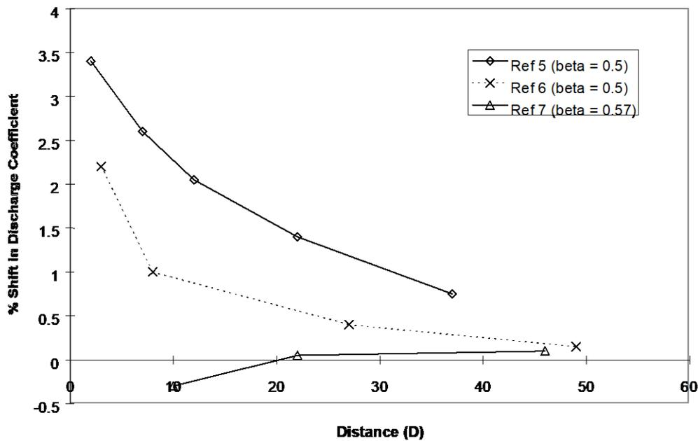
**Figure 8. Measured Shifts in Discharge Coefficient of an Orifice Plate Downstream of a Twisted Double Bend**
