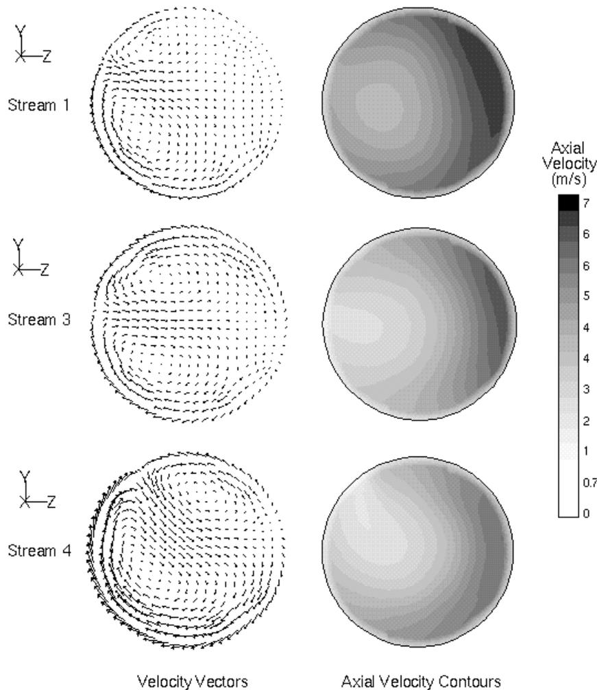
**Figure 5. Predicted Flow Behaviour 1.5m Downstream of the Header with Streams 1, 3 and 4 on-line**
