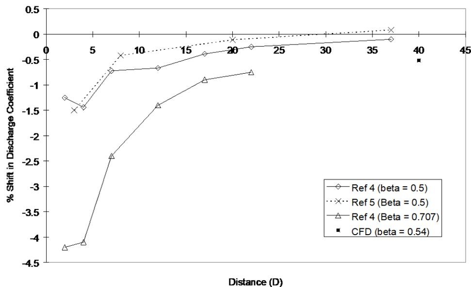
**Figure 7. Comparison of Measured and Predicted Shifts in Discharge Coefficient of an Orifice Plate Downstream of a Single Bend**
