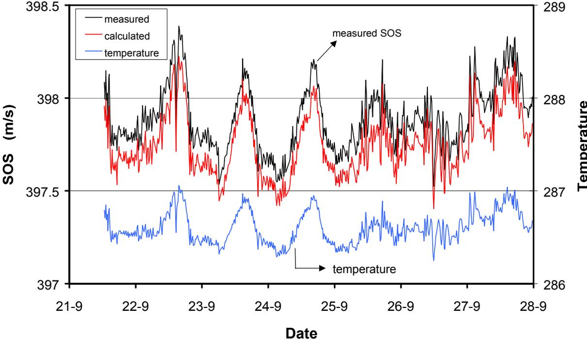
**Figure 5. The measured and calculated speed of sound and the measured temperature, data collected over 7 days (Station D).**
