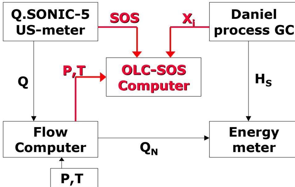
**Figure 1. OLC-SOS set-up during field tests at Gasunie metering stations**
