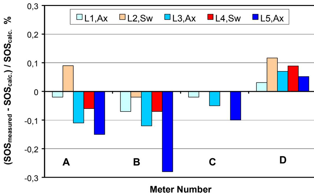
**Figure 2. The differences between measured and calculated speed of sound for the individual chords of 4 different ultrasonic flow meters.**
