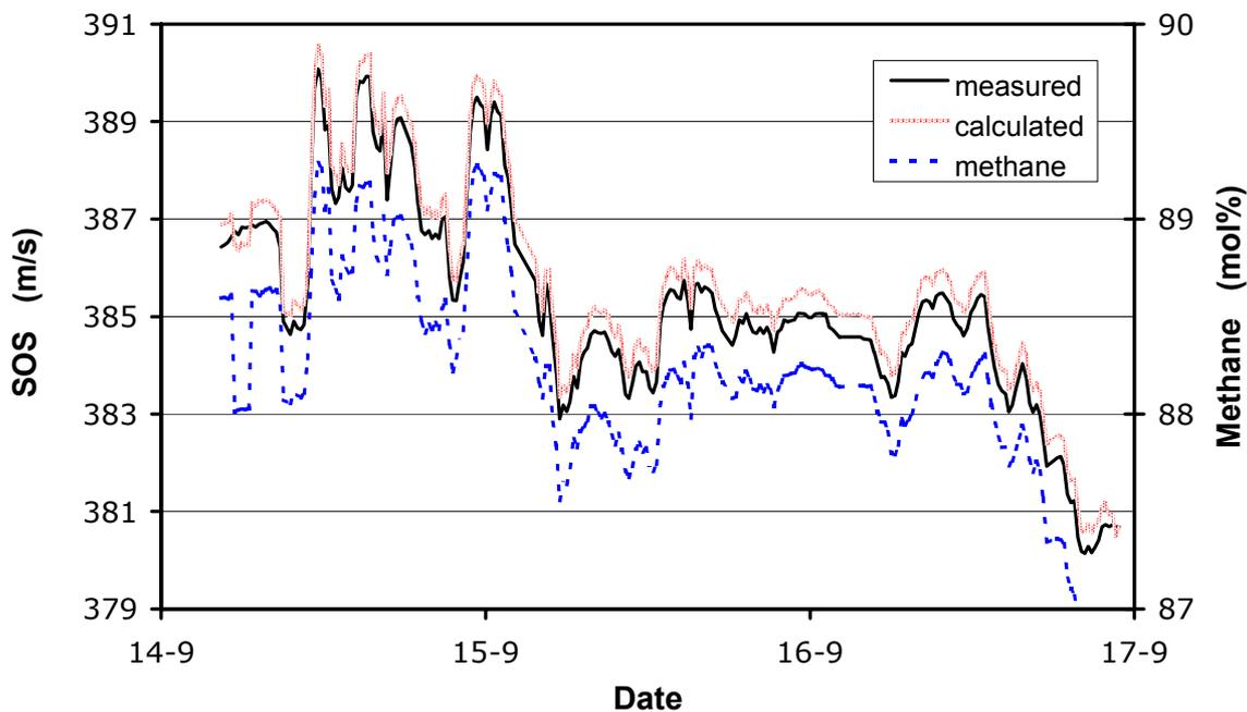
**Figure 3. The measured and calculated speed of sound and methane concentration collected during 3 days at Station B.**
