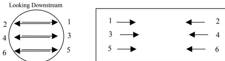
Fig. 3 - Layout of Paths Used in the USZ-08-6P Flowmeter.
