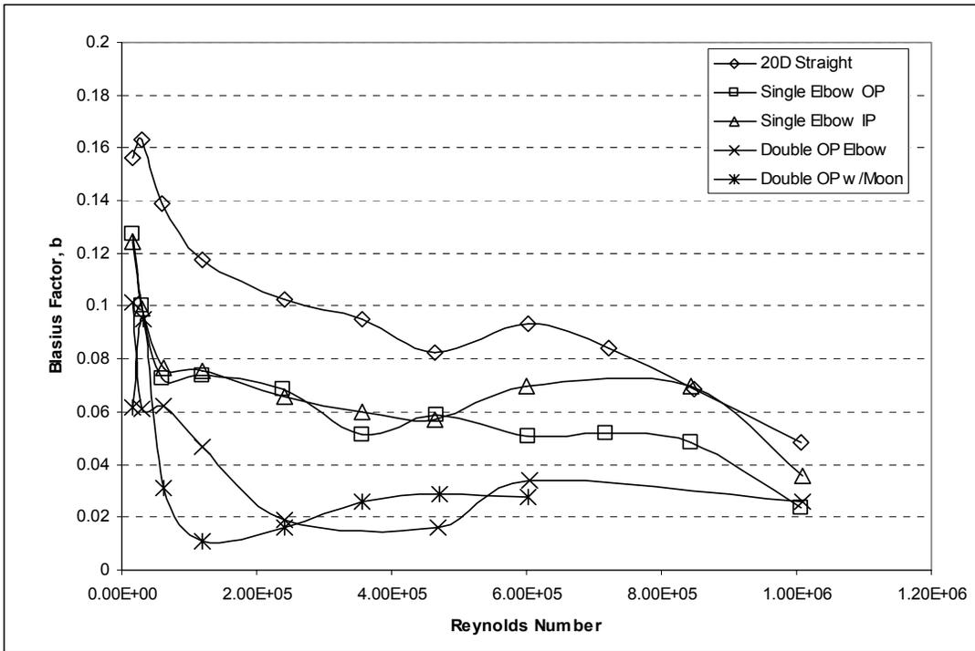
Fig. 4 - Blasius Profile Factor for Five Standard Meter Installations
