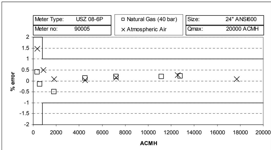
Fig. 11 – Comparison between Air and Natural Gas Calibration of 24 Inch Meter
