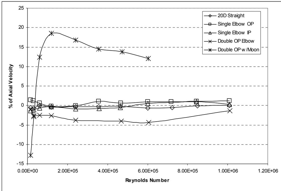
Fig. 7 – Cross-Flow Generated by Five Standard Meter Installations
