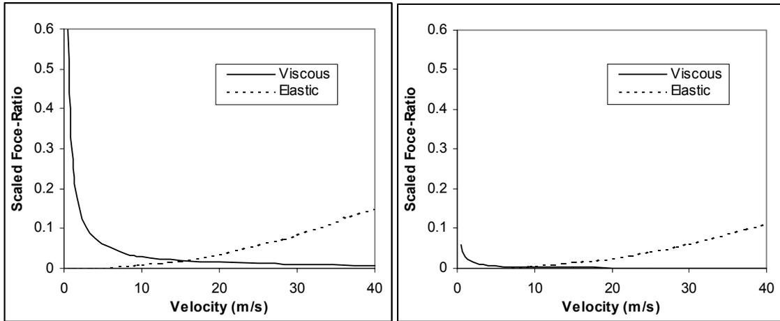
Fig. 1 – Viscous and Elastic Force Ratios for a) Air and b) Natural Gas
