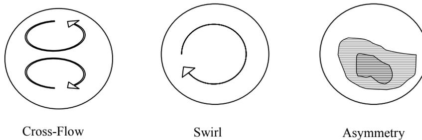
Fig. 2 - Types of Disturbed Flow
