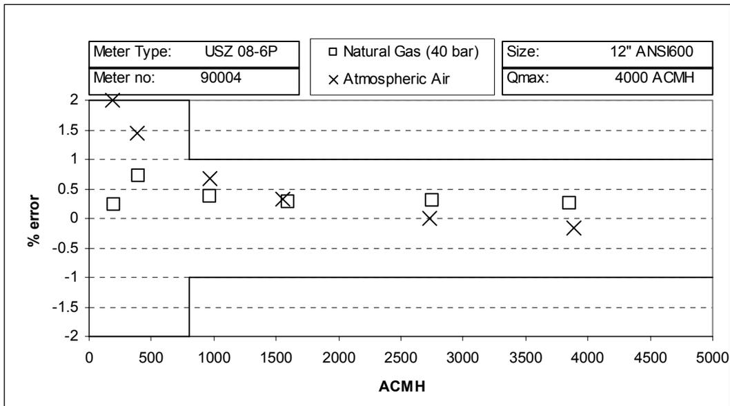
Fig. 10 – Comparison between Air and Natural Gas Calibration of 12 Inch Meter
