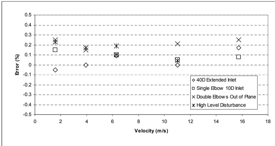
Fig. 8 – Error Shifts for Four Installations in 10 bar Natural Gas
