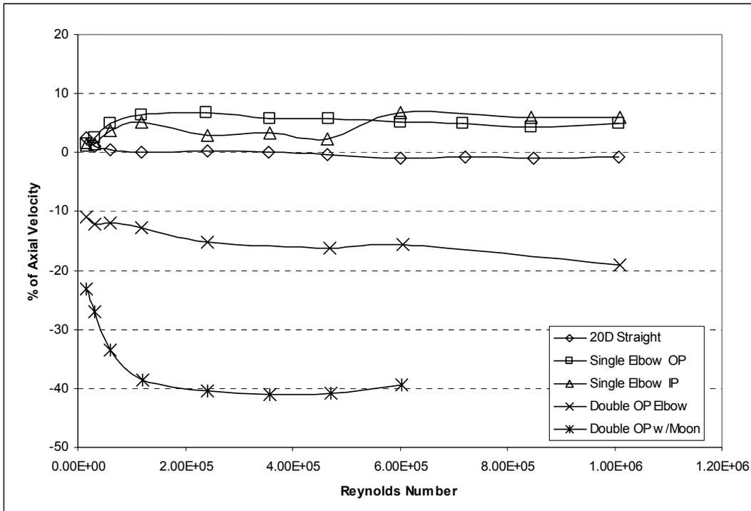
Fig. 6 – Swirl Generated by Five Standard Meter Installations
