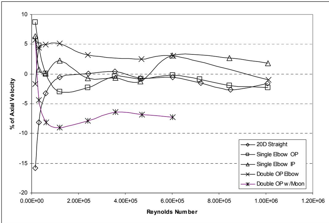
Fig. 5 – Asymmetry of the Flow Profile for Five Standard Meter Installations
