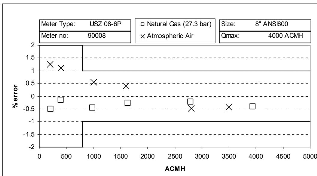
Fig. 9 – Comparison between Air and Natural Gas Calibration in 8 inch size
