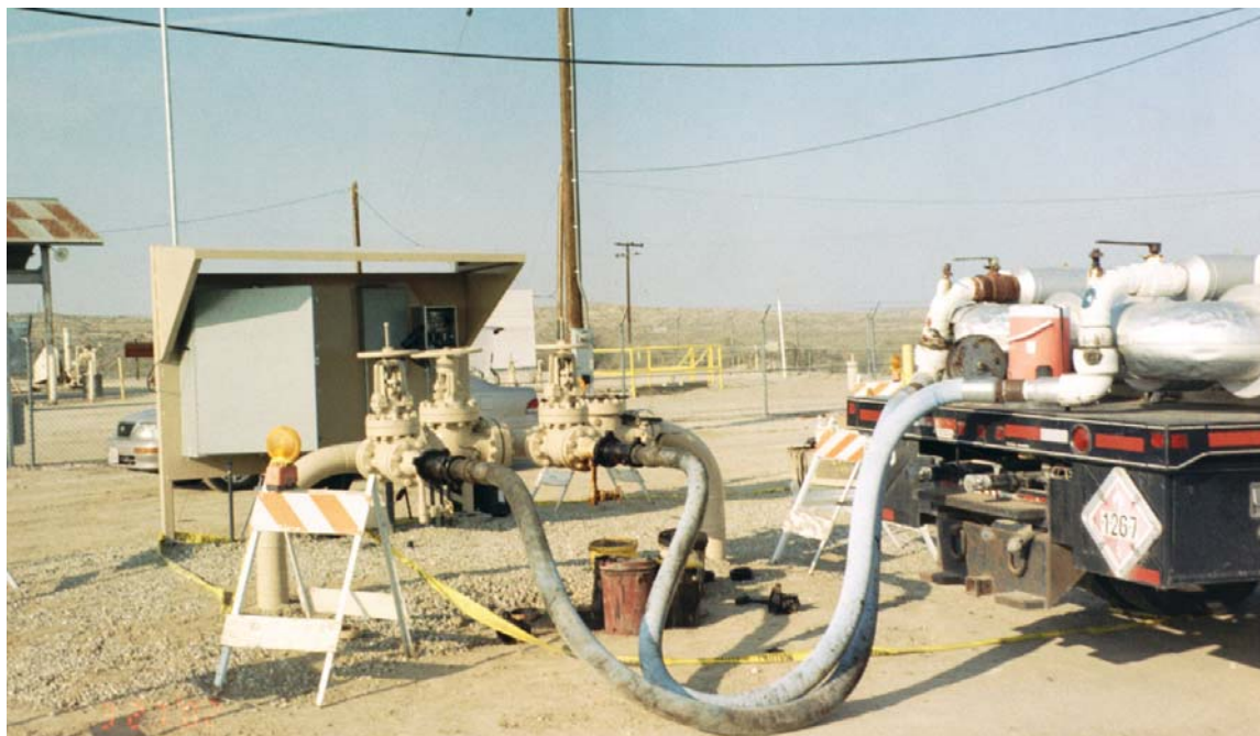
Figure 5: Compact Prover Test Configuration
