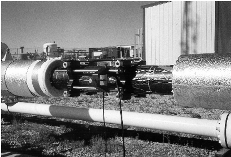
Fig. 4 – 10.2-cm Ultrasonic Clamp-on Meter Installed at CEESI Wet Gas Flow Loop
