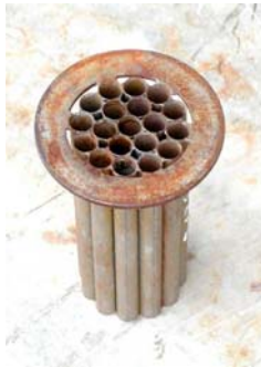
Fig. 12 - 4" 19-tube bundle flow conditioner
