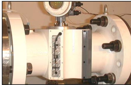
Fig. 7 – A side of 4 transducers and cables without cover
