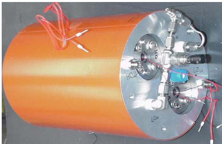
Fig. 8 - The high and low pressure VOS-meter in one housing made of aluminium and surrounded by a heat tracing.
