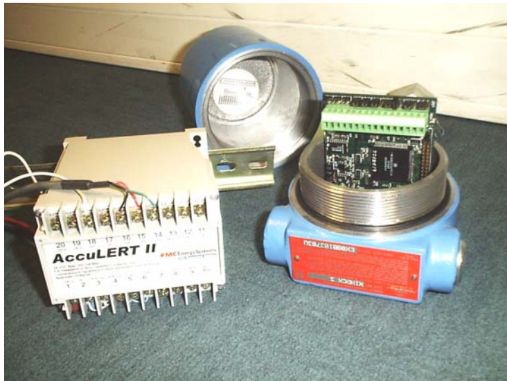
Picture 2 - The AccuLERT II (DIN rail and explosion-proof versions) (Gaz de France)
