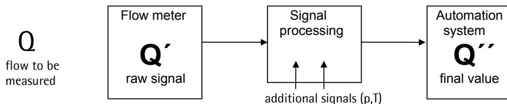
**Figure 1** The flow measurement chain
