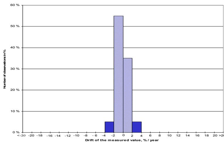
Fig. 3. Instability in natural gas flow measurements observed as the change of the total error / year. The number of observations is 20.
