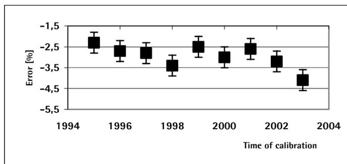
Fig. 5. Calibration history of a liquid gas flow measurement. The uncertainty bars represent the repeatability of the calibration.
