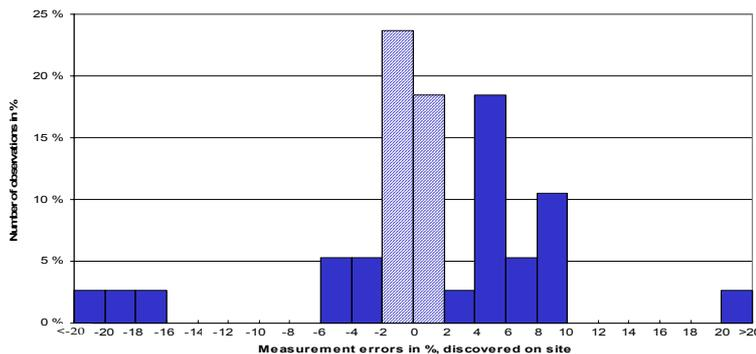
Fig. 4. Total measurement errors in oil flow measurements observed in first time field calibrations. Number of observations is 34.
