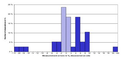
Fig. 4. Total measurement errors in oil flow measurements observed in first time field calibrations. Number of observations is 34.
