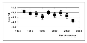
Fig. 5. Calibration history of a liquid gas flow measurement. The uncertainty bars represent the repeatability of the calibration.
