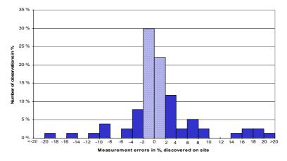
Fig. 2. Total measurement errors in natural gas flow measurements observed in first time field calibrations. Number of observations is 77.
