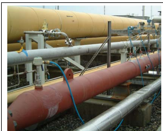
FIGURE 7:- DUPLICATE DUALSTREAM II METER INSTALLED AT K-LAB
