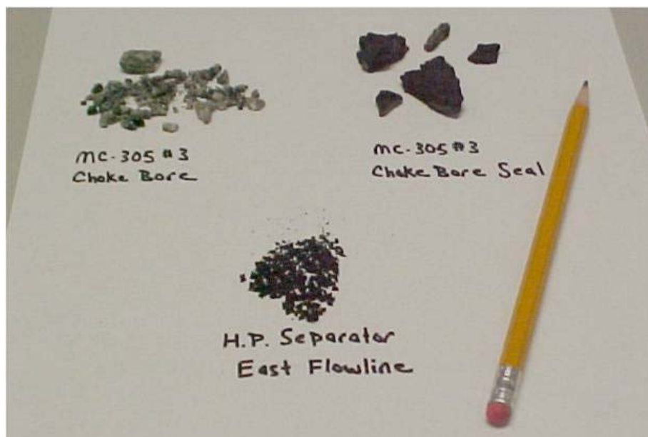
Figure 8. Scale found inside flow line of Well 305-3 after intervention.
