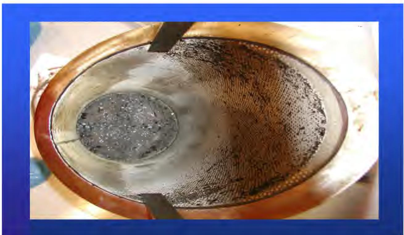
**Figure 5** Flow Shift From Clogged Filters
