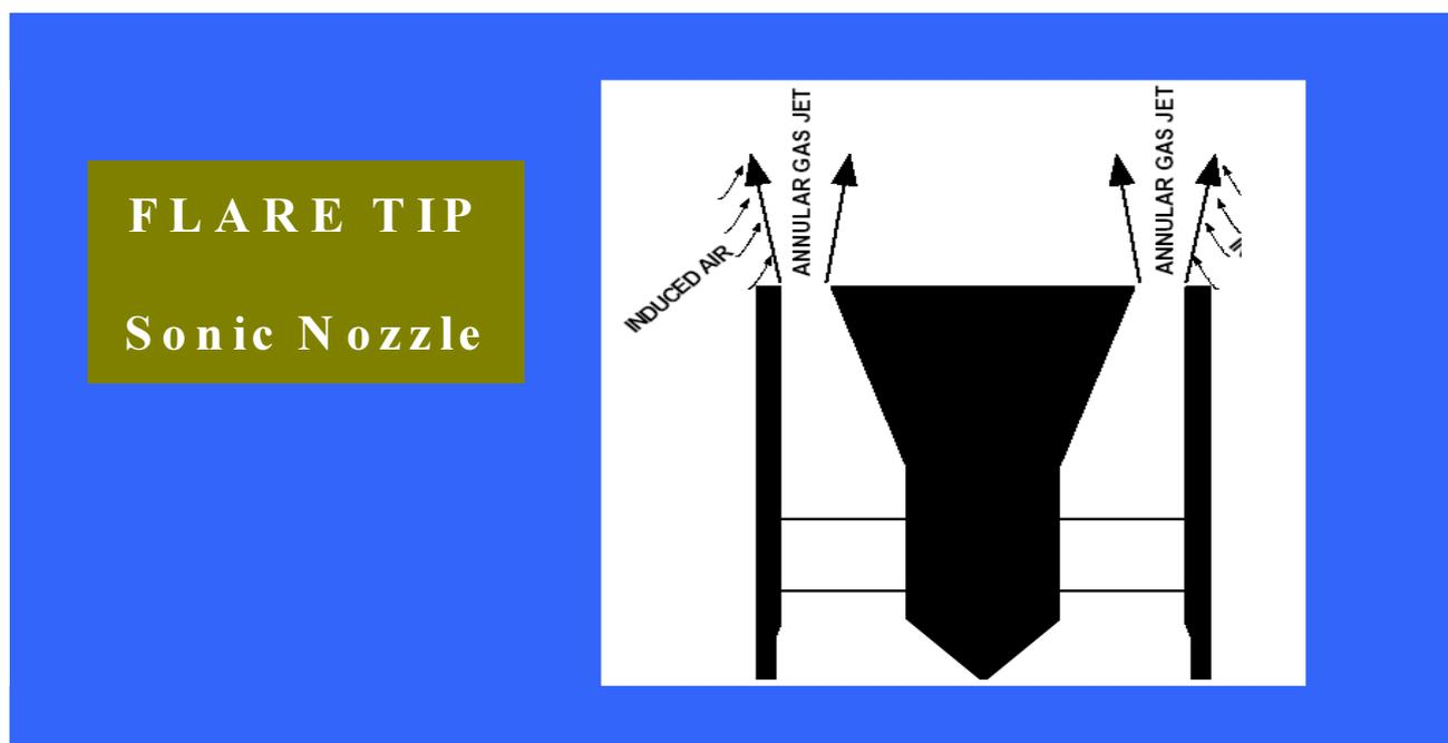
Figure 1. Flare Tip Sonic Nozzle
