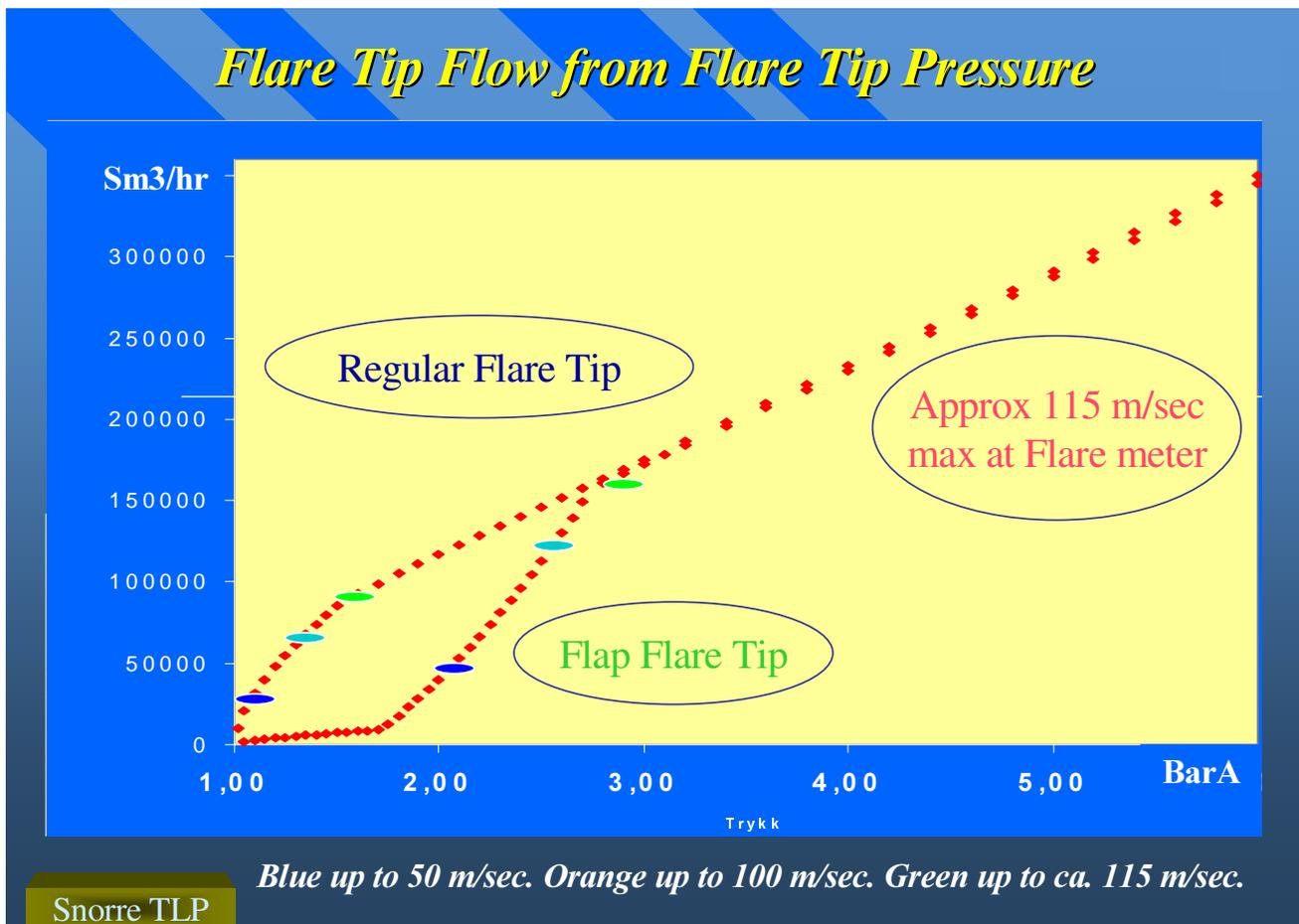
Figure 6. Snorre TLP Flap Flare Tip Performance compared with Regular Flare Tip
