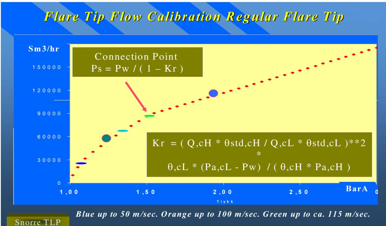
Figure 5. Flare Tip Critical Nozzle calibration Critical Pressure Point
