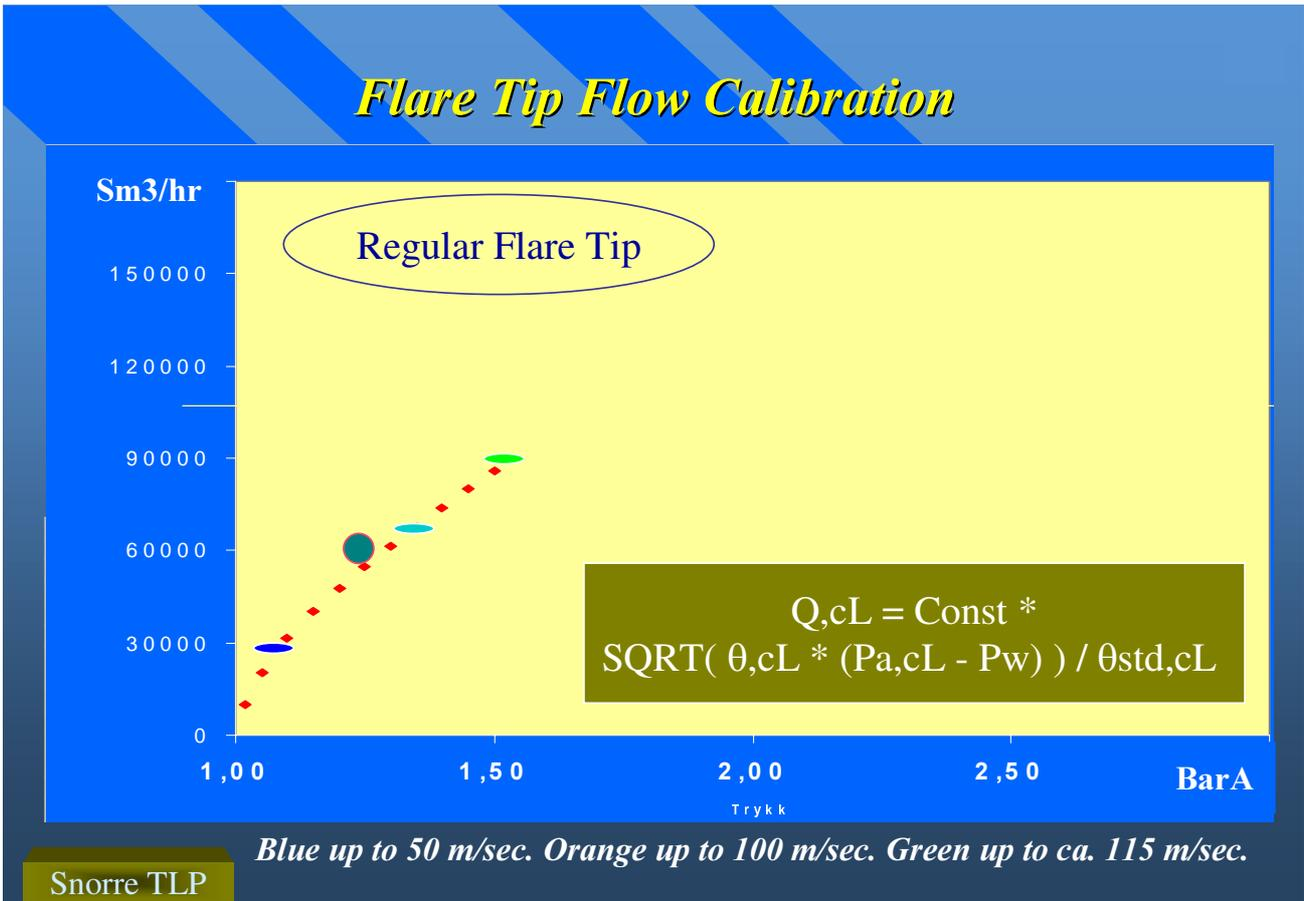
Figure 4. Lower velocity end calibration of Flare Tip Critical Nozzle
