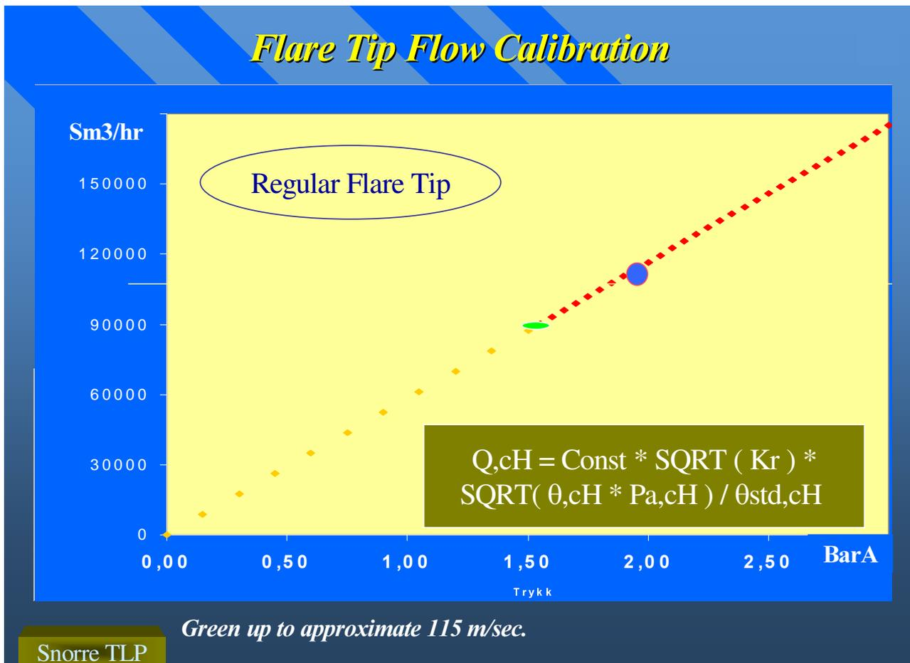
**Figure 3. Velocity of sound limited high end calibration of Flare Tip Critical Nozzle**
