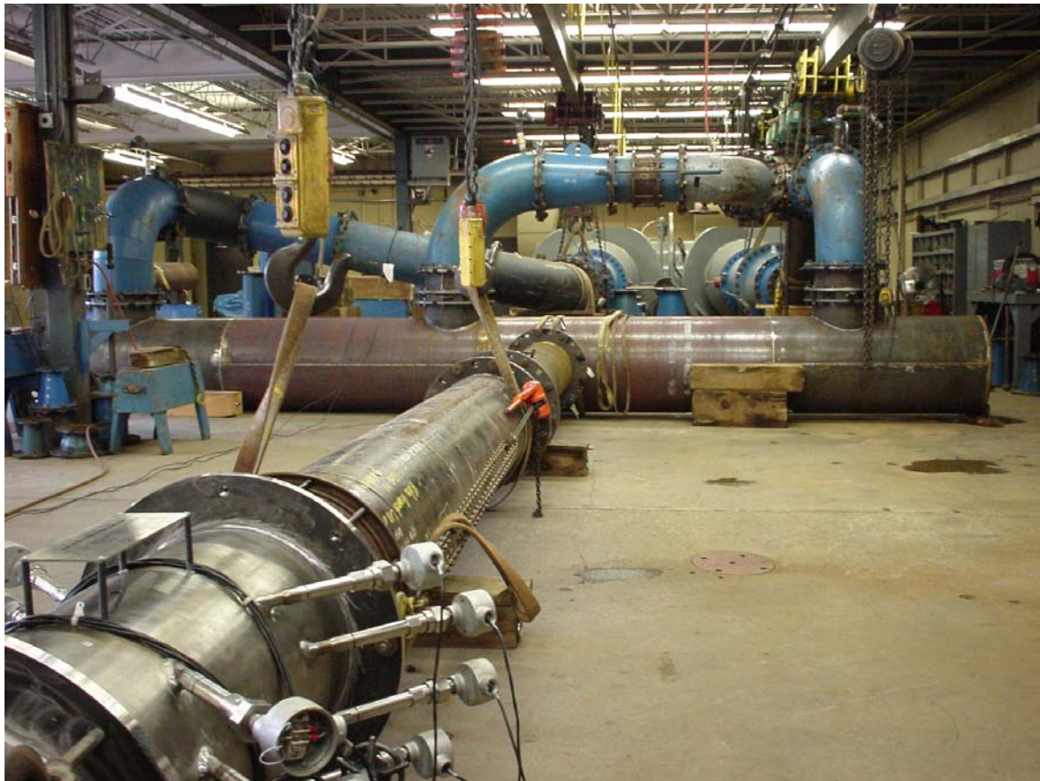
Figure 1 Calibration of a Chordal UFM for Nuclear Service in a Full Scale Hydraulic Model
