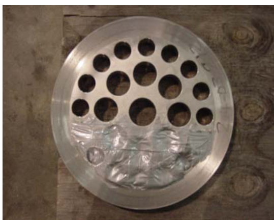
Figure 15 – Blocked Flow Conditioner
