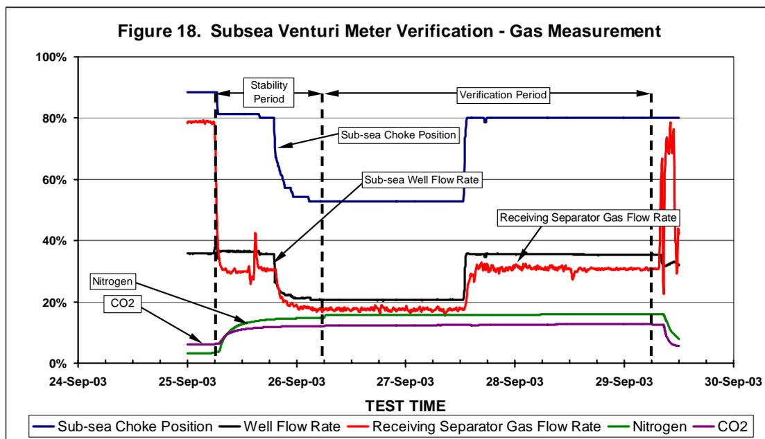
Figure 18 also shows the choke settings for the test field well. The field production follows these settings quite precisely, and the field flow rate was very stable.
