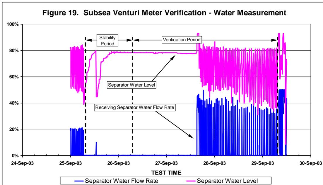
Figure 19 above shows the plot of the water production during the verification. The bottom trace shows the water flow rate; the upper the variations in separator interface level. The spike at about mid-day on 25 September corresponds to the water being drained prior to the test. The separator was operated in batch flow mode.
