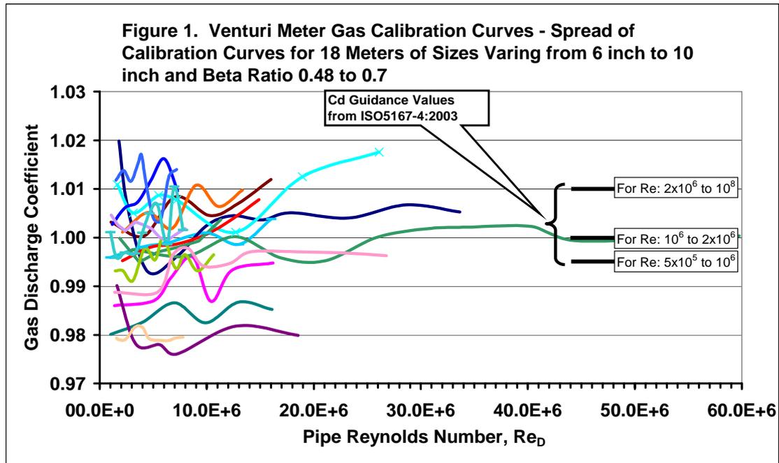
Figure 1 above shows similar gas calibration curves for 18 Venturi meters with diameters ranging from 6 to 10 inches and beta ratios ranging from 0.48 to 0.7. The meters were calibrated at the Advantica Flow Centre at Bishop Auckland on sales-quality natural gas. For the meters calibrated, the variation in discharge coefficients is about 4%. The curves themselves are evidently not linear, and many show sharp kinks. This confirms findings by Jamieson et al (Ref [1]).
