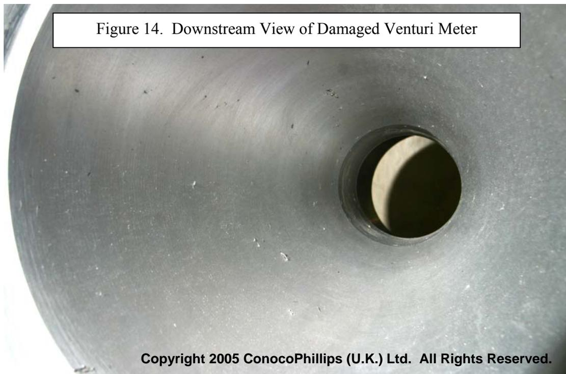
Our original plan was to re-machine the damaged section of the meter, recalibrate it and return it to service. However, we decided to determine the effect that the damage
