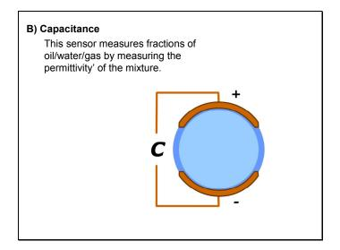
Functioning as a capacitor, the MPFM 1900VI measures the permittivity (dielectric constant) of the oil/gas/water mixture. The permittivity is different for each of the three components in an oil/gas/water mixture, and the permittivity of the mixture is therefore a measure of the fractions of the different components.
