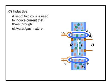
When the liquid is water-continuous, the mixture conductivity of the oil/water/gas flow is measured by an inductive sensor. Magnetic coils are used to induce a current through the liquid inside the sensor
