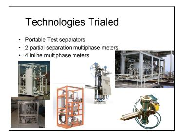
In a trial phase in 1999 – 2000 a total of 6 different multiphase meters were installed offshore in separate periods of time. Each meter was tested over a period of 1 - 3 months. During this time, the meters were tested over a selection of wells and compared with the test separator.
