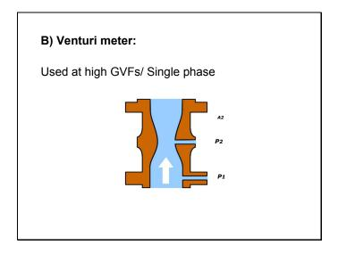
In many applications, the combination of a mass based Venturi meter and a volume based cross-correlation is beneficial. At very high GVF's (typical around 95-99%) the cross correlation technique may not work accurately due to lack of dynamics in the measurement signals from the capacitance/inductive sensor. A typical example would be annular flow where the gas mainly travels in the center of the MPFM sensor with the liquid concentrated along the walls of the sensor.
