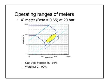
The meters where installed close to wellhead, and saw direct well stream. The wells are gaslifted, which causes a very high GVF. The typical gas void fraction is 85 – 95%. In addition many wells were had heavy slugging, as normally occurring in gas lift wells.
