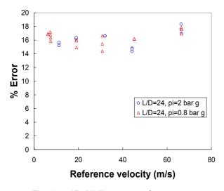
Fig. 14 – IR4MKII meter performance at the L/D=24 injection position at pi = 0.8 bar g and 2 bar g
