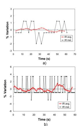
Fig. 17 – Instantaneous and average velocities logged at: a) 7 m/s, b) 67 m/s
