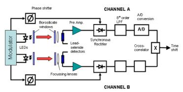
Fig. 4 – Schematic of the electronics of the IR4MKII meter
