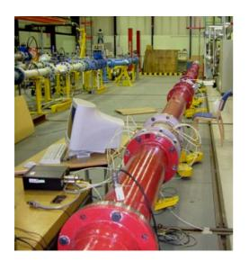
Fig. 9 – Photo of IR4MKII meter installed in NEL's fanline facility
