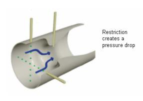
Fig. 1 – Schematic of a differential pressure device
