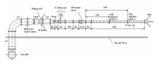
Figure 8 - Installation of the IR4MKII meter in NEL's atmospheric fanline (note: flow is from right-to-left)
