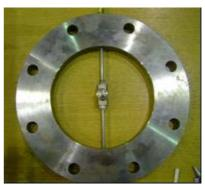
Fig. 10 – Water injection system and photo of nozzle mounted in carrier ring
