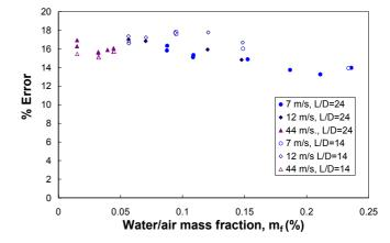
Fig. 12 – Meter error vs. water-to-air mass fraction, m<sub>f</sub>, at three discrete velocities
