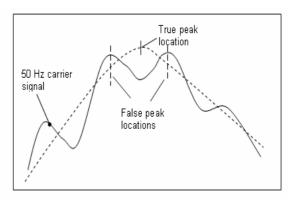
Fig. 19 – Schematic of the correlation peak as modulated by the carrier signal
