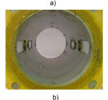
Fig. 7 – IR4MKII meter spool and internal view
