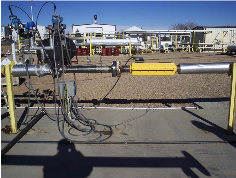
Figure 2: Picture of DP plus SONAR Configuration installed on 4 inch Multiphase Loop at CEESI (Flow is from right to left)
