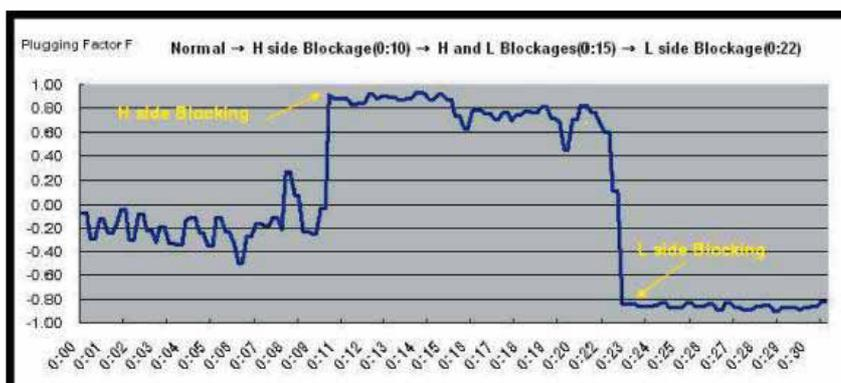
Fig.2 Blocking diagnostics for water flow
