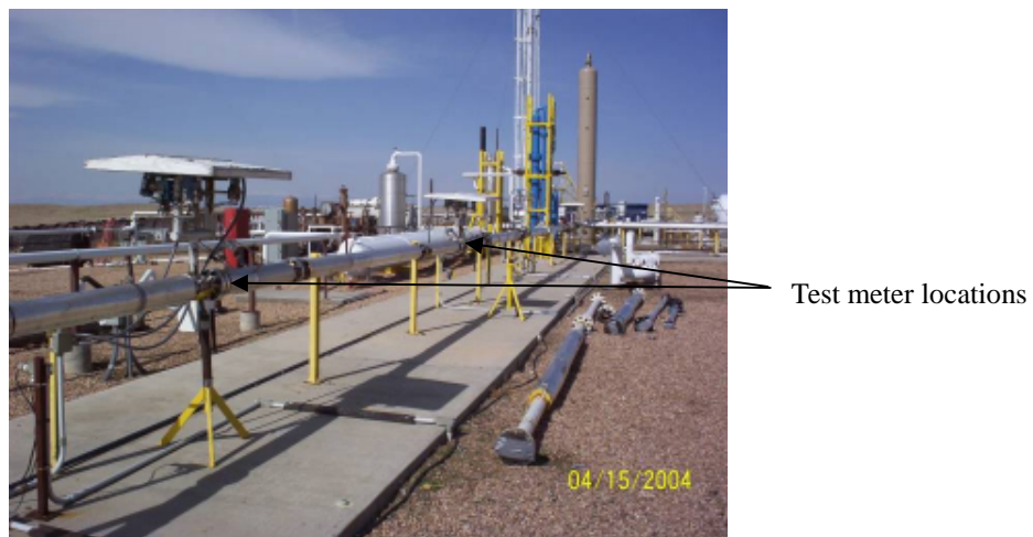
Fig. 1 Test setup at CEESI wet gas testing facility
