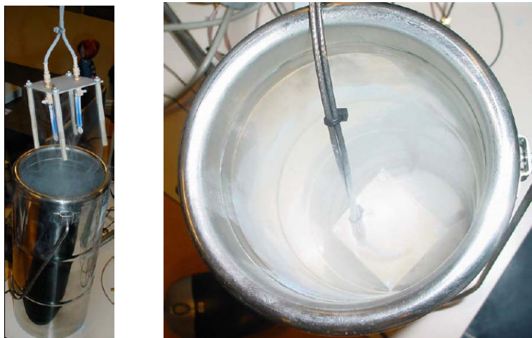
Figure 1 Set up for piezo tests at liquefied nitrogen (-196 [°C]).
