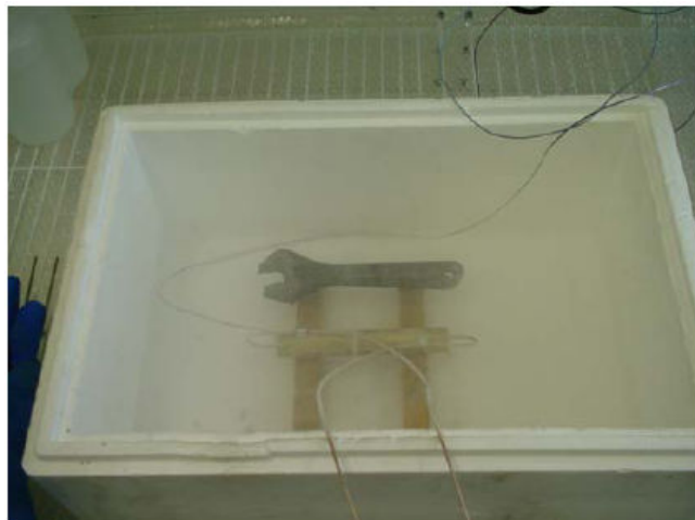
Figure 6 Test object with final transducer construction, submerged in liquefied Nitrogen at -196 [°C].
