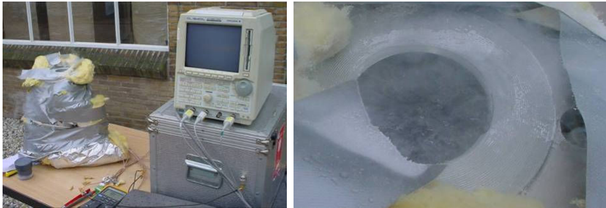
Figure 9 Static flowmeter tests on liquefied Nitrogen. Left hand figure: set up. Right hand figure: Flowmeter filled with Nitrogen.
