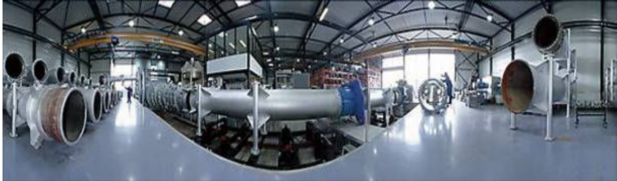
Figure 10 Fisheye picture of the water calibration facility at KROHNE Altometer, The Netherlands. Maximum flow rate 3 \cdot 10^4 [m 3 /h], max. diameter 3.2 [m]
