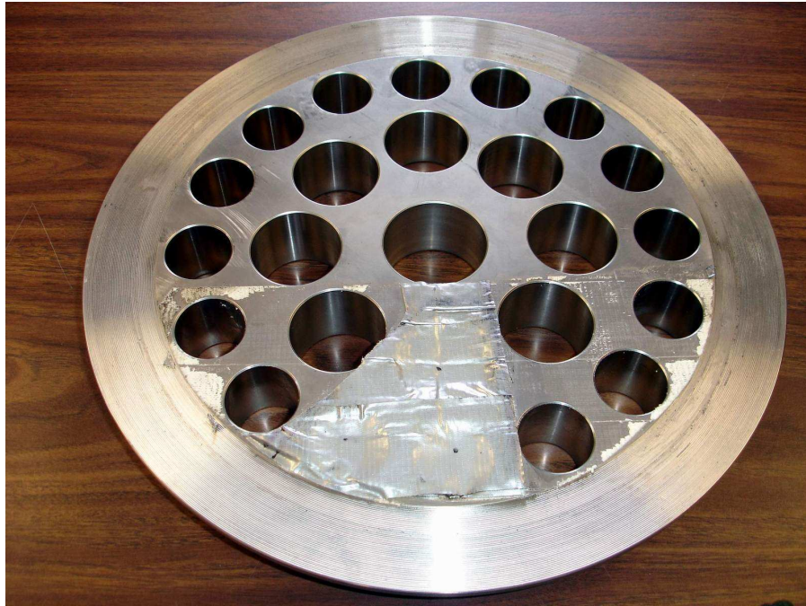
Figure 9: 12-inch CPA with 3 Holes Blocked
