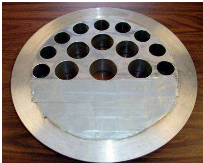
Figure 6: 12-inch CPA with 40% Blockage
