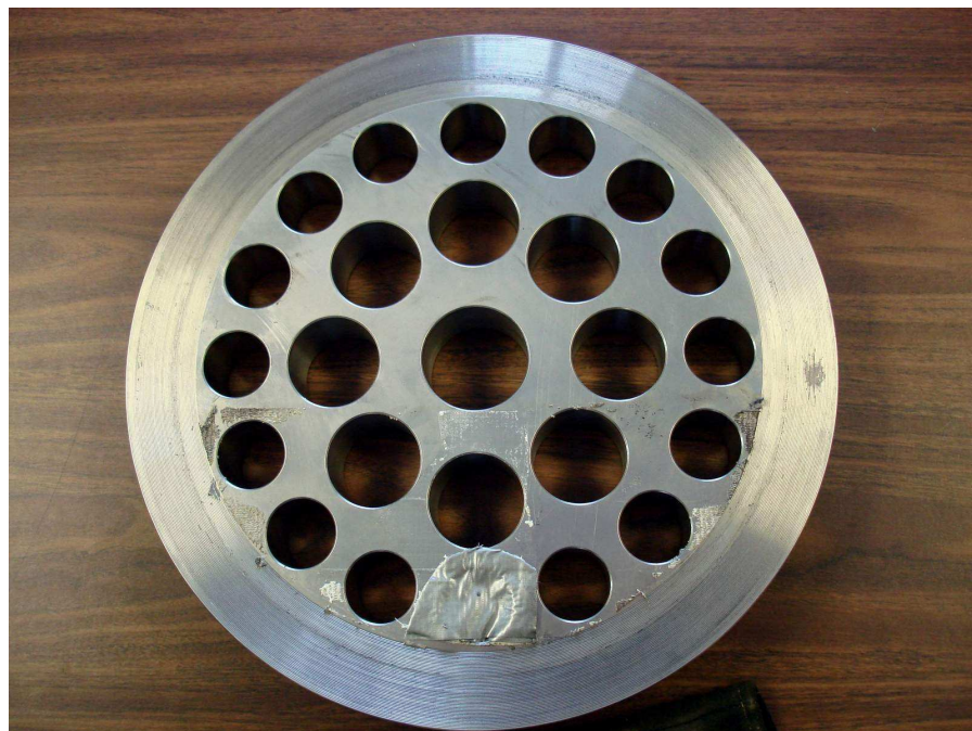
Figure 12: 12-inch CPA with 1 Hole Blocked
