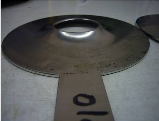
Fig 12. Severely buckled orifice plate.
