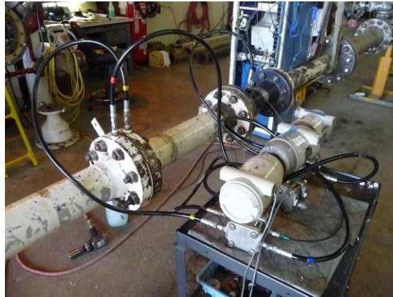
Fig 4. Flange installed plate with air flow.
