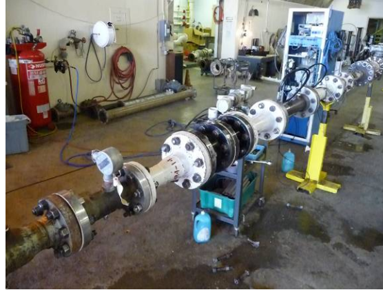
Fig 40. 3" Swirl Generator + Expansion 9D up
