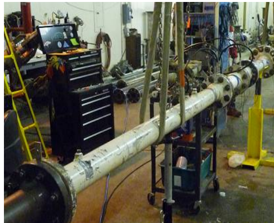
Fig 27. Meter installed with upstream HMOP.
